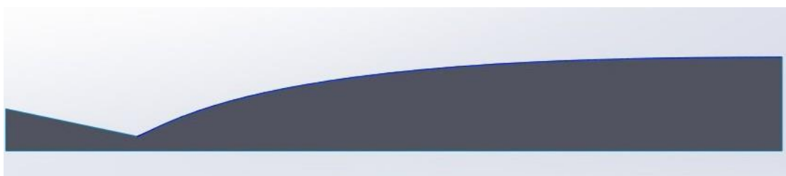
Figure 4.3: 2D contour of Nozzle after the points were imported in a CAD software
