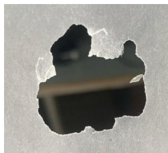
Figure 5.9: Single layer tracing paper burst pattern
