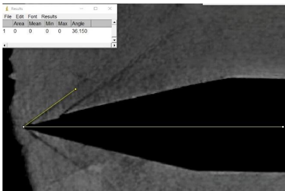
Figure 5.24: shock wave at upper part of wedges Aluminium Foil (4:3)
