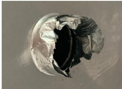
Figure 5.10 Aluminum foil as diaphragm when oil between the two layers.
