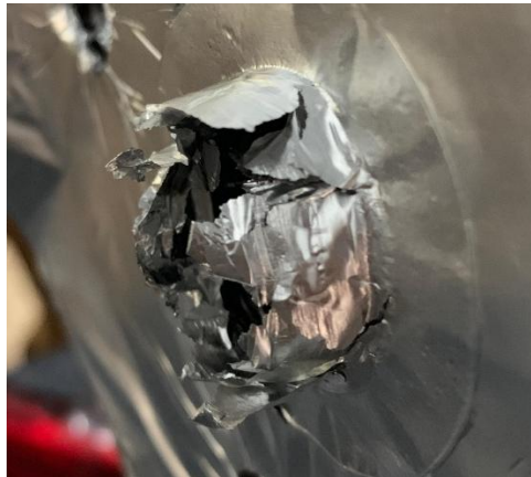
Figure 5.11: Aluminium diaphragm Burst Pattern between tube and nozzle
