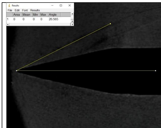
Figure 5.18: shock wave at upper part of wedges. Tracing Paper Thick (2:1 Ratio)
