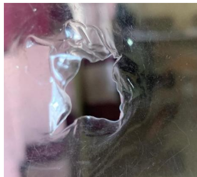
Figure 5.12: Nylon sheet as primary diaphragm of shock tube
