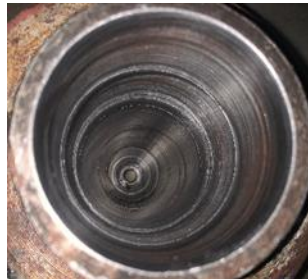
Figure 4.5: Nozzle inside surface after polishing
