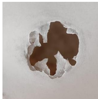
Figure 5.8: Burst pattern of three layers of Tracing Paper as Diaphragm
