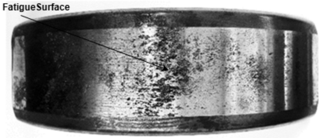
Figure 2.7: Material Fatigue of a Rolling Bearing [13]
