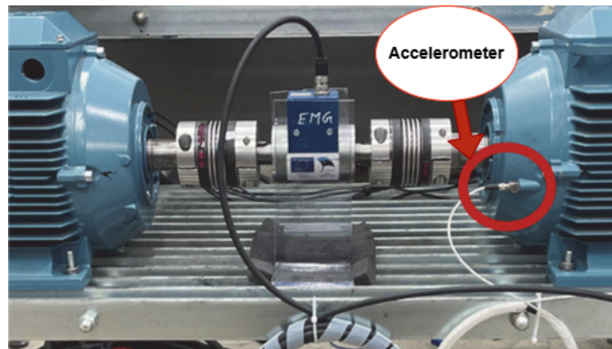
Figure 3.4: Placement of Triaxial Accelerometer [49]
