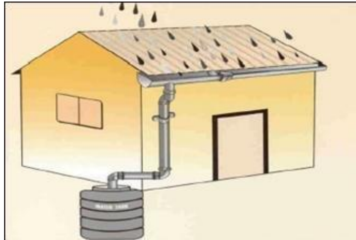
Fig.2-14: Roof dependent RWH-system
