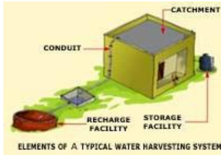
Fig.2-13: Common Rainwater Harvesting System's components (rainwaterharvesting.org)
