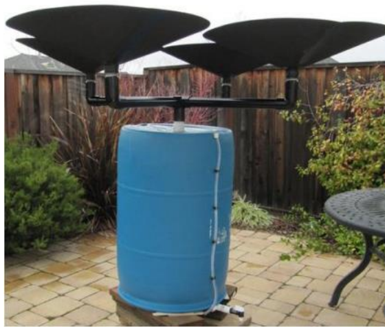
Fig.2-16: Example of Rain Saucer design (Hofer, 2014)
