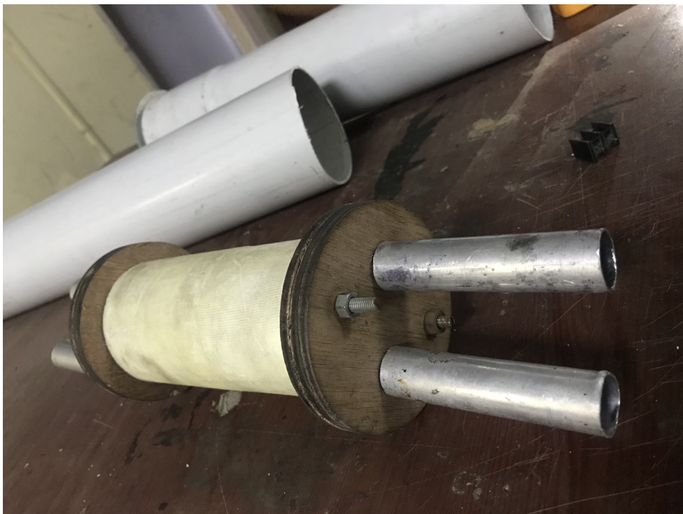
Figure 6.3: Electronics Bay and Ejection Canister
