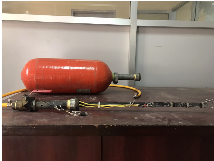
Figure 4.14: Crawford Strand Burner
