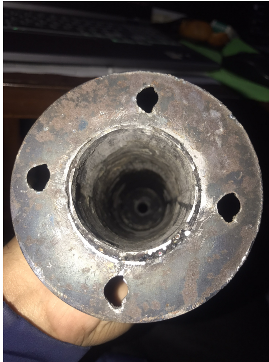
Figure 4.6: Stainless Steel Tube as Combustion Chamber
