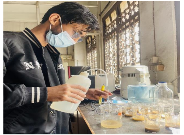
D. Soil PH Measurement
