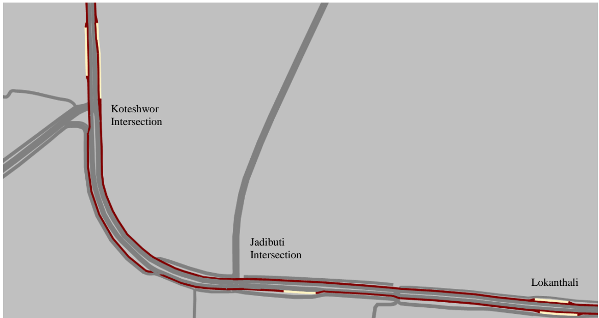
Figure 4.16: Layout showing the exclusive bus lanes in scenario S2
