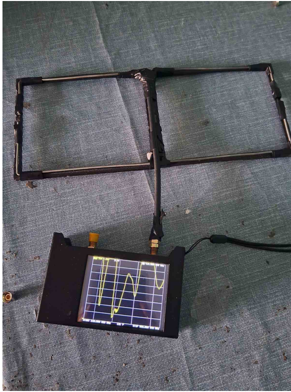
Figure 4.2: Moxon Antenna 4th iteration, tested on a Nano VNA depicting SWR
