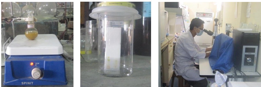
Plate 4: (a) Fractionation of CEE, (b) TLC of CEE, (c) Counting of parasite using hemocytometer
