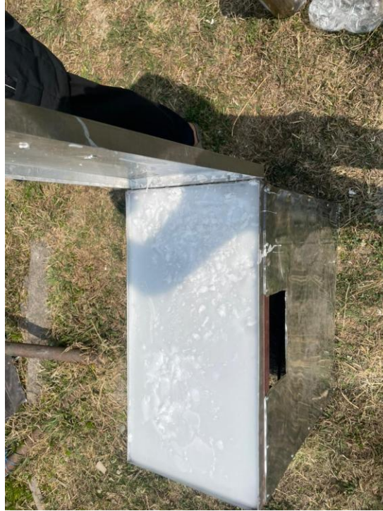
Figure 29: Poured Paraffin in Cavity(1)
