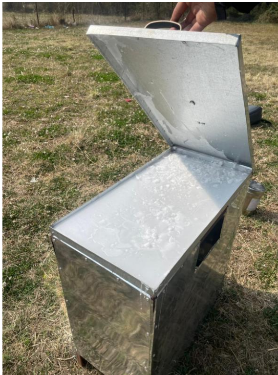
Figure 30: Poured Paraffin in Cavity(2)
