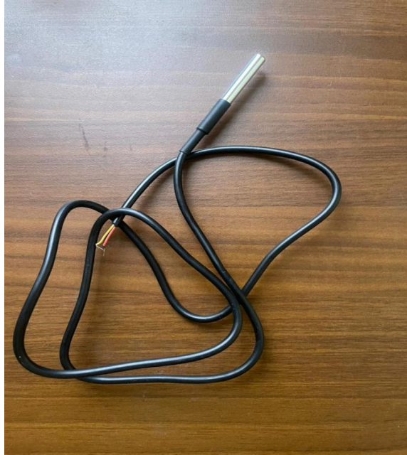
Figure 27:DS18B20 temperature sensor
