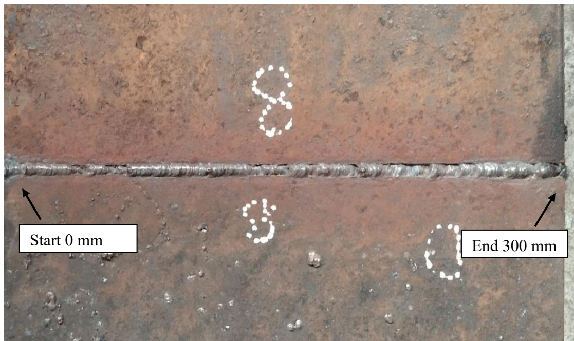
Figure 4.11: Photographic representation of root penetration at 8 mm root opening
