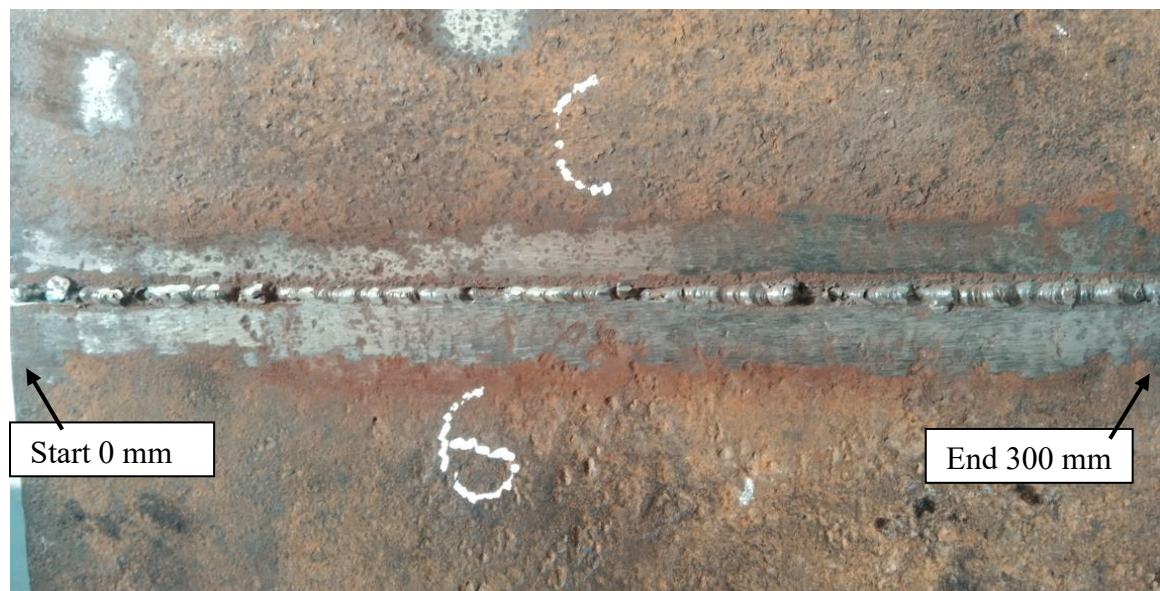
Figure 4.9:Photographic representation of root penetration at 6 mm root opening
