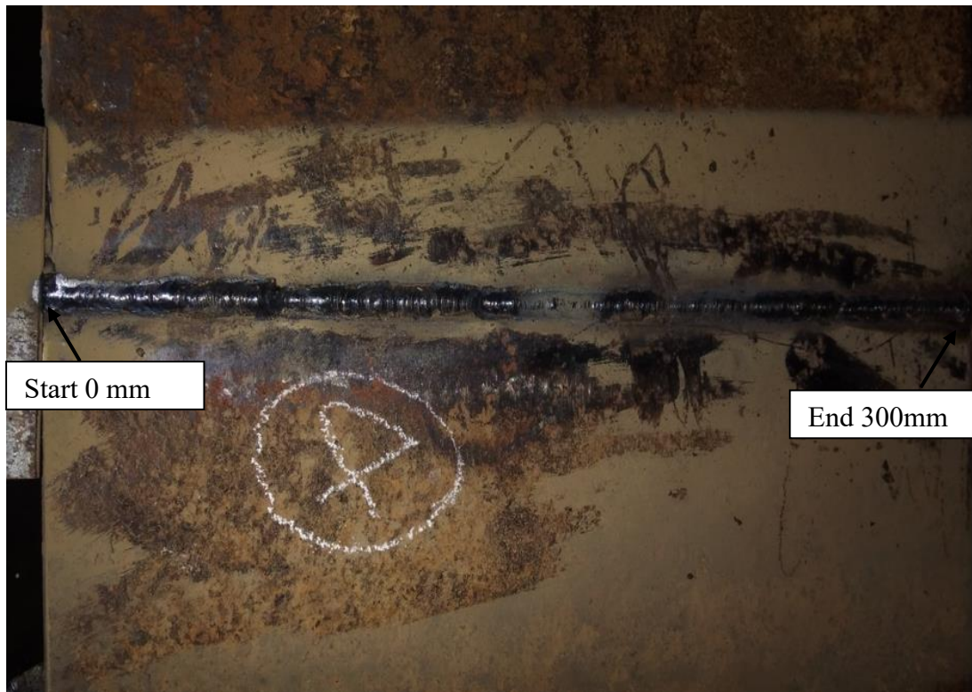
Figure 4.7:Photographic representation of root penetration at 4 mm root opening
