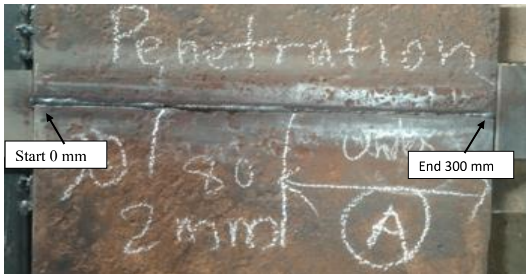
Figure 4.4: Root penetration at 2 mm root opening
