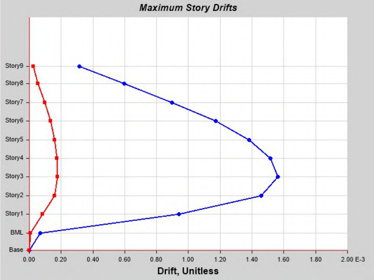
Fig. Maximum Story drift in EQx direction
