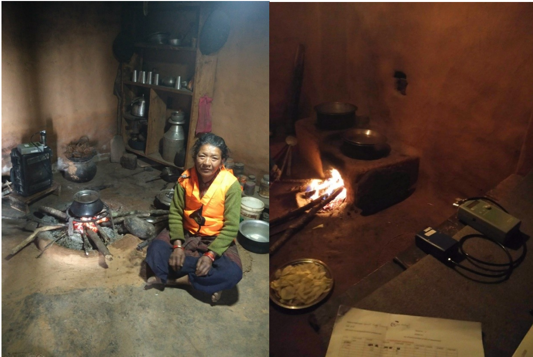
Figure 3.4: a) TCS (open fire); b) ICS (two-pot mud type)
