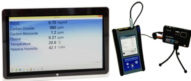
Figure 3.1: IAQ probe with interface
