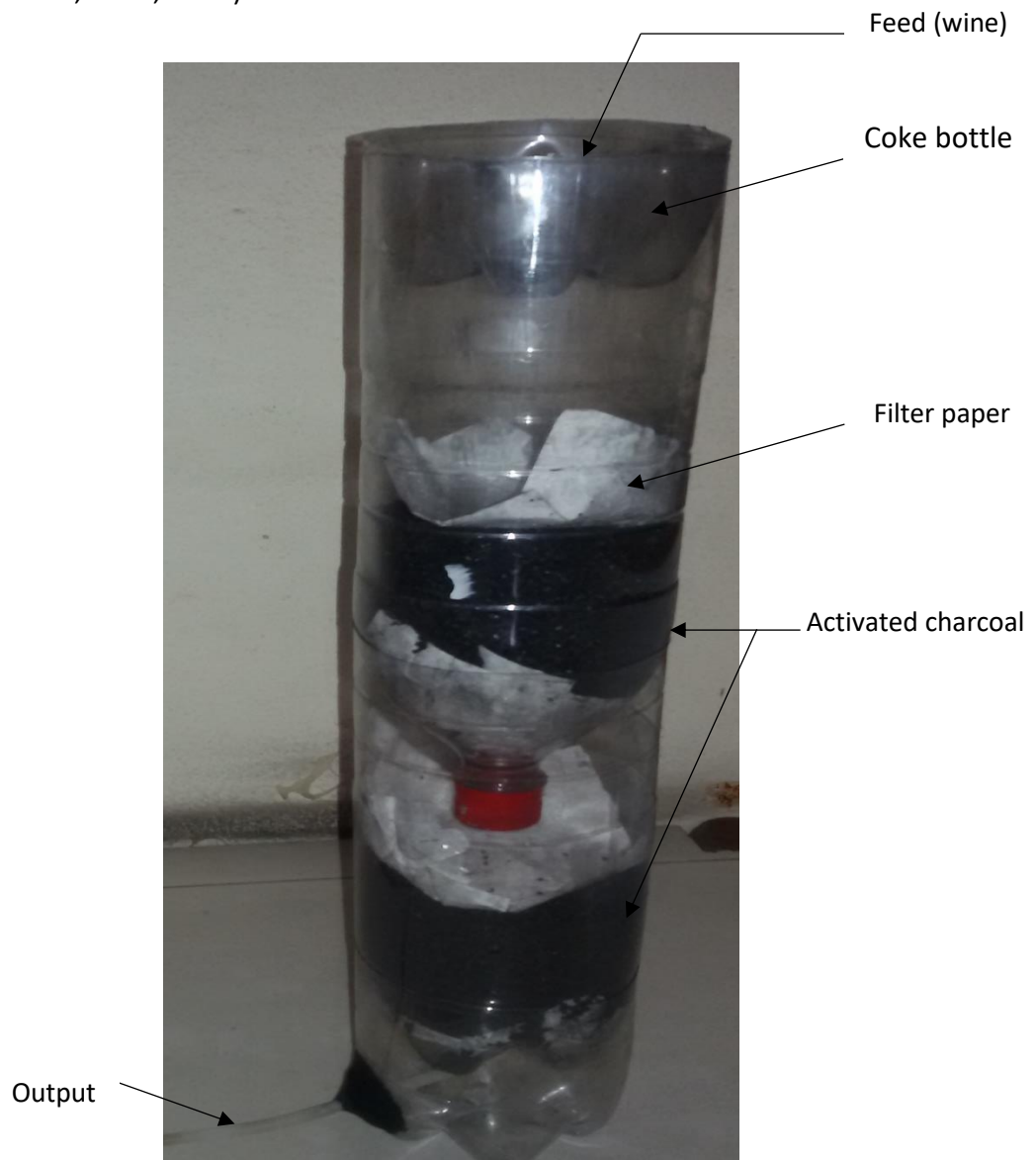
Fig. 3.2 General setup prepared for charcoal clarification.
