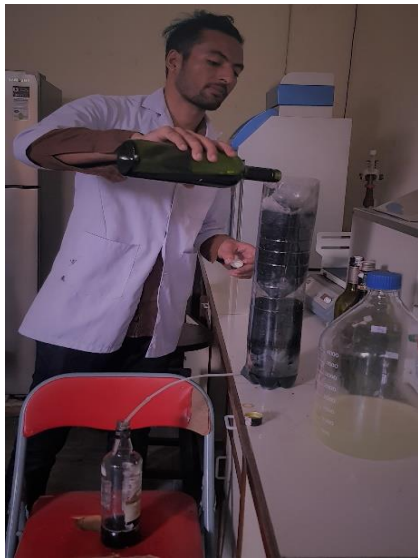
Photo 15 Sake filtration through activated charcoal
