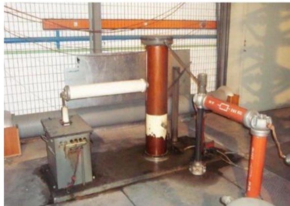
Figure 3.6: Experimental setups of Greinacher
