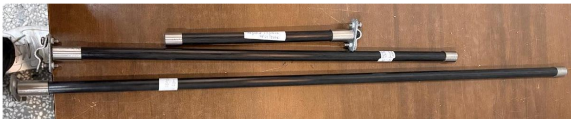
Figure 3.14: 25cm Insulating Standoffs
