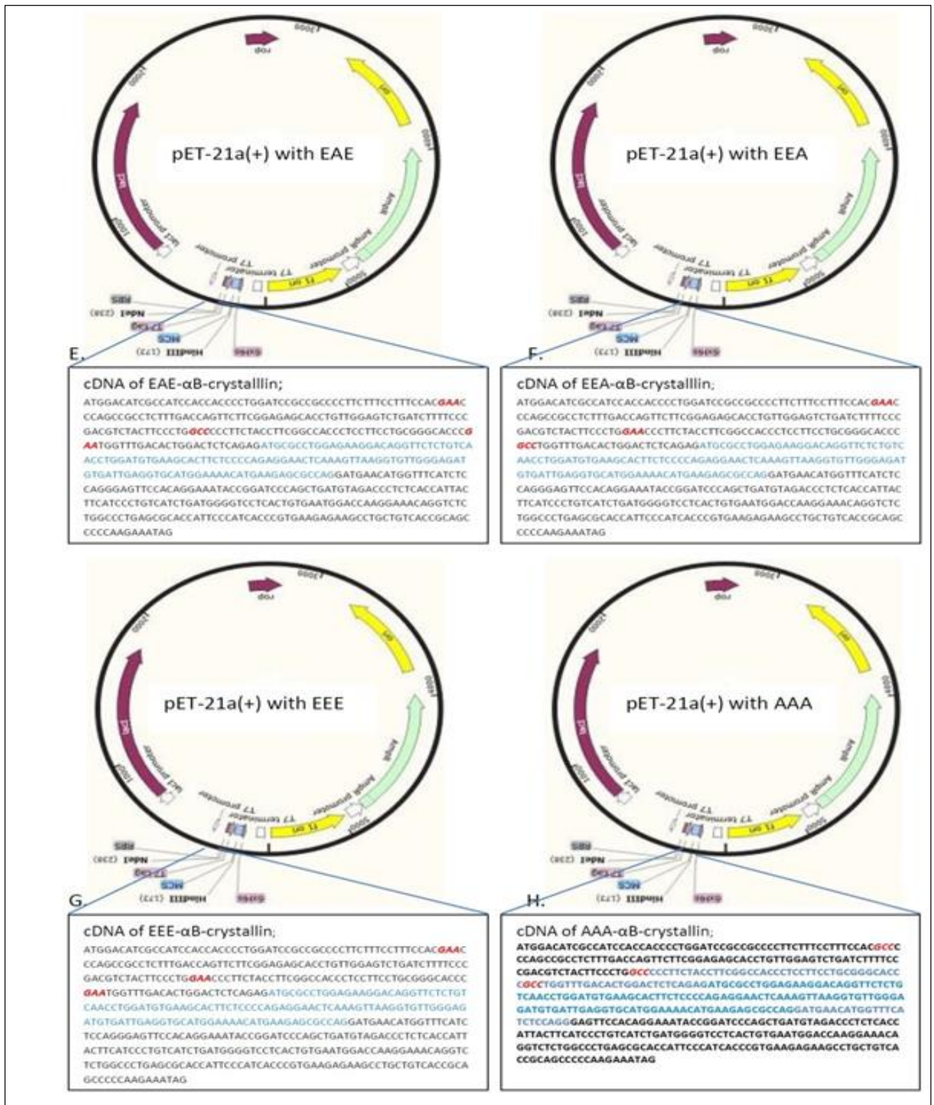
Figure 5: Schematic diagrams (A-D) of gene construct for mutants WT- \alpha B crystallin protein coding gene in pET21a expression vector cloned in NdeI and Hind III site. Site of mutation and crystallin domain are shown in red and blue color respectively.
