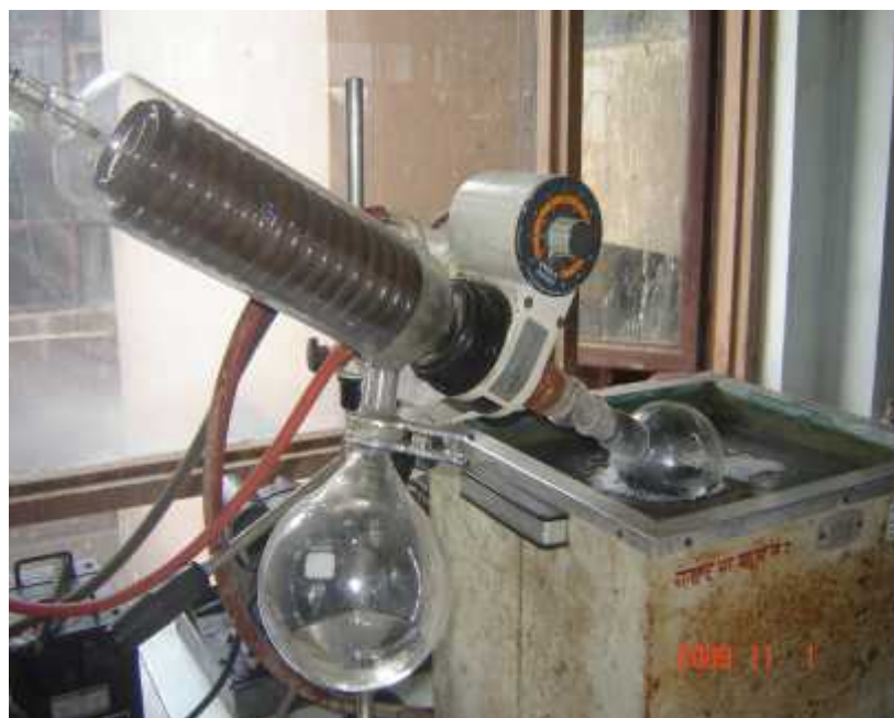
Fig. 4.4: Drying extract with the help of Rotatory Vacuum Evaporator.
