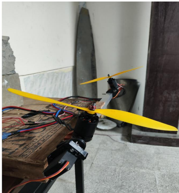
Appendix 15 Motors Orientation Check in Opposite Direction for Moment Generation.
