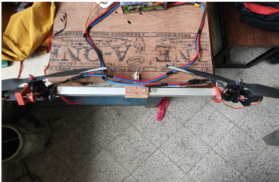
Appendix 13 Complete Experimental Setup for Thrust Calculation at Different Tilt Angles.
