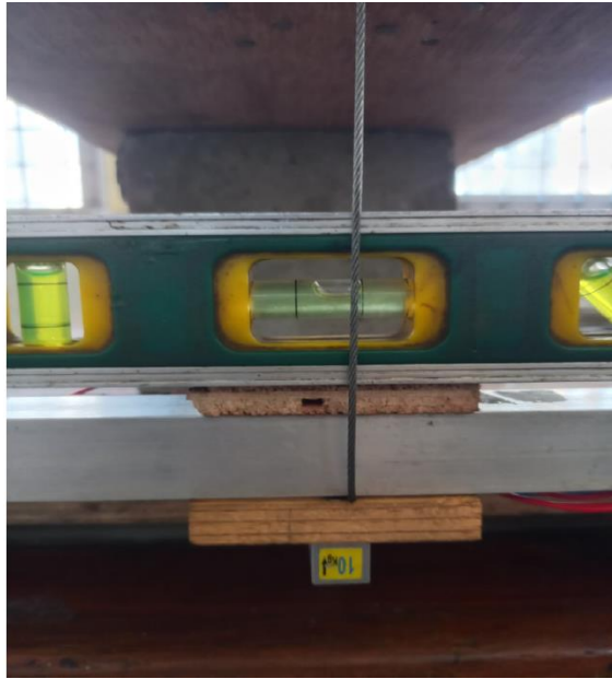
Appendix 16 Leveling of Setup Before Deflection Check of the Setup.
