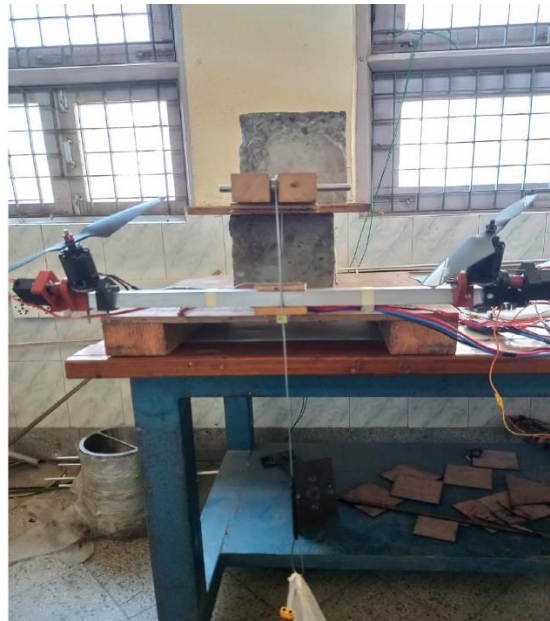
Appendix 11 Loadcell Calibration Setup.
