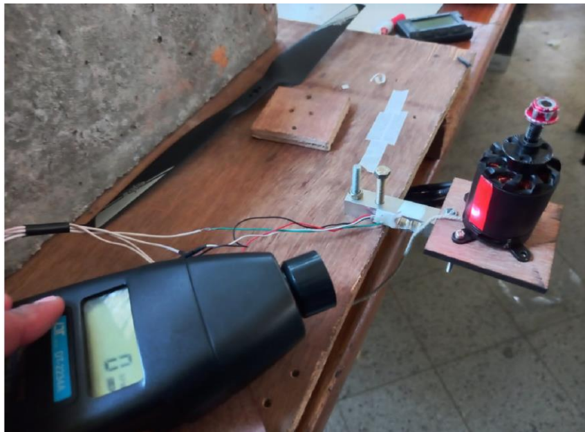
Appendix 17 Tachometer Setup for RPM Calculation for Experiments.
