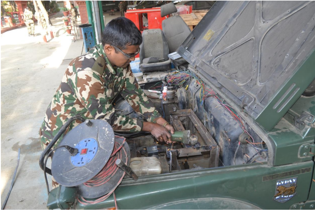
Preparation of New mounts for Battery
