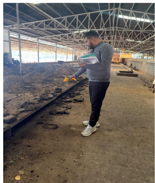
Measurement of surface temperature
