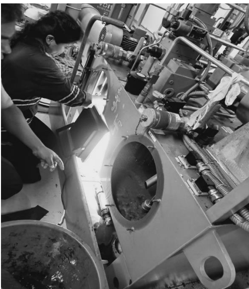
Oil Sump Tank Cleaning
