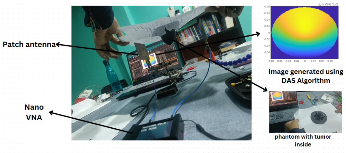
Figure 4.16: Reconstructed image from the DAS algorithms, showing tumor localization within the phantom. The image, presented in its non-normalized form, highlights the tumor's present high dielectric contrast.
