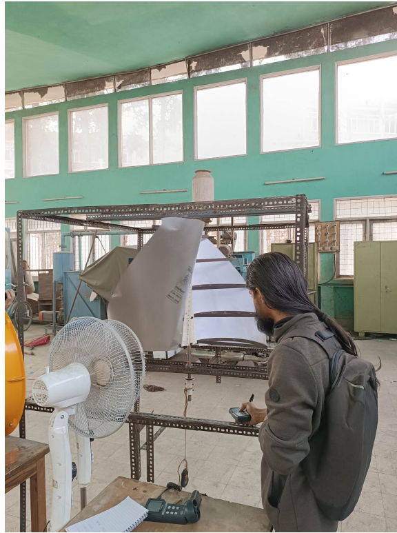
Figure 5.12: Measuring RPM of Turbine
