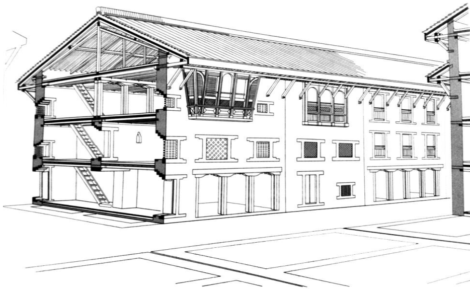
Figure 21: Sectional view of typical Newari house
