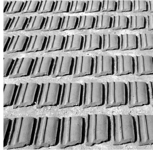
Photo 2:Clay Roofing tiles
