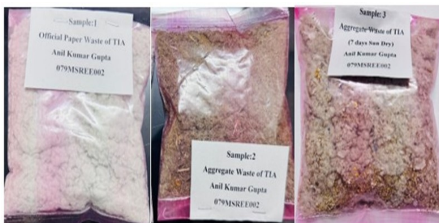
Figure 4.3: Sample Prepared for GCV Testing at RETS (NAST)
