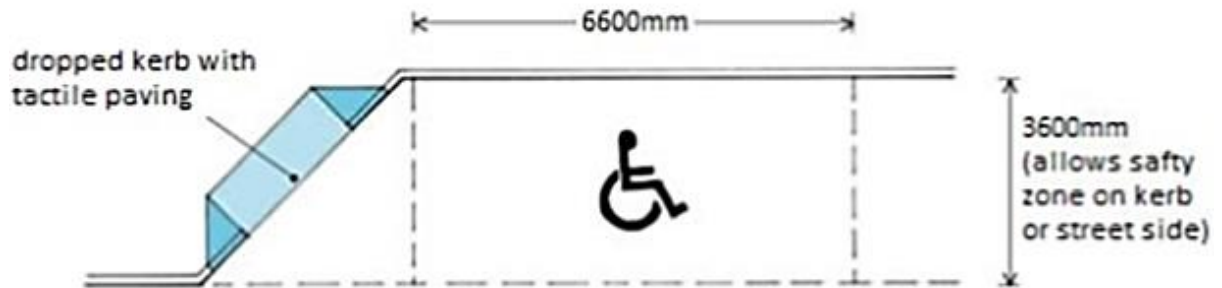
Figure 6. Plan of street accessible parking with kerb ramp (Centre for accessible environments and RIBA 2004)
