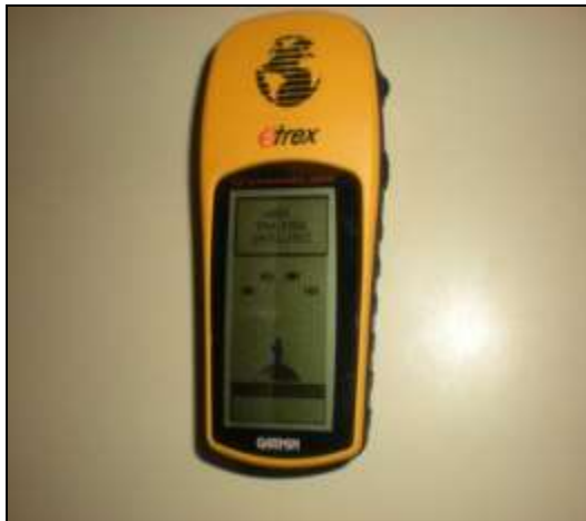
GPS used for boundary survey
