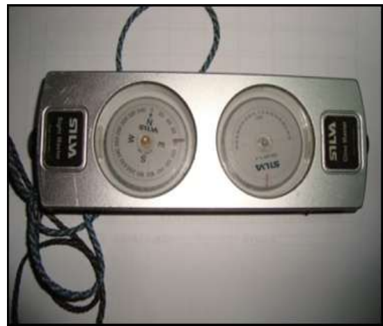
Clinometer for measuring treeheight
