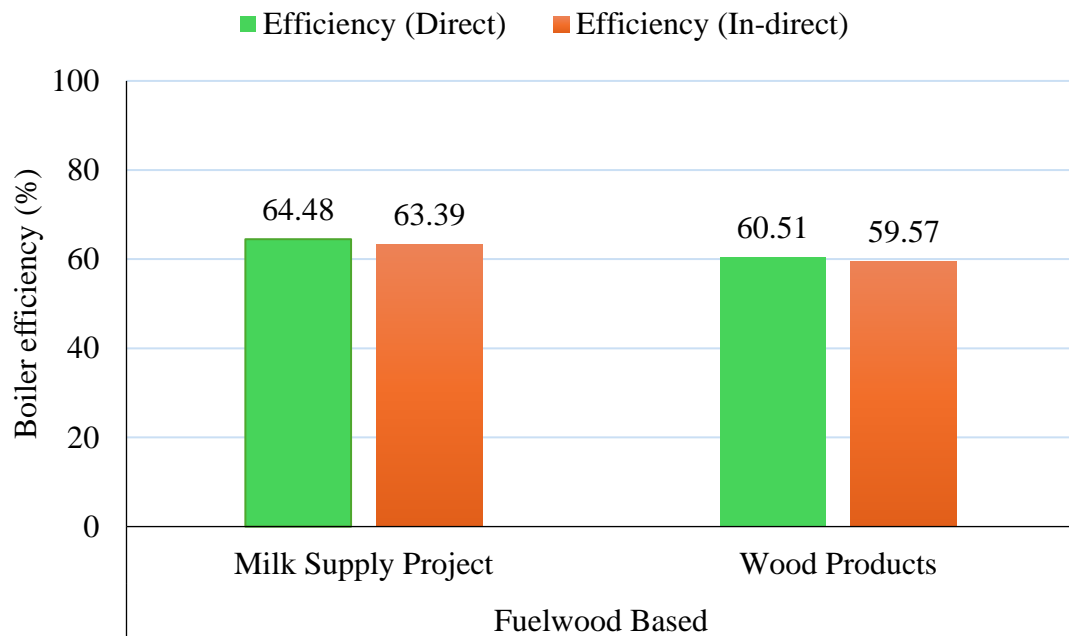
Figure 4.12 Direct and Indirect Efficiency of the fuelwood-based boilers
