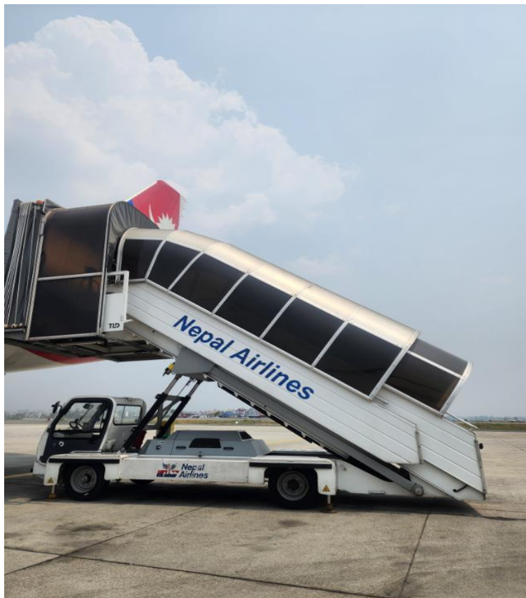
Figure B.4: Passenger Stairs
