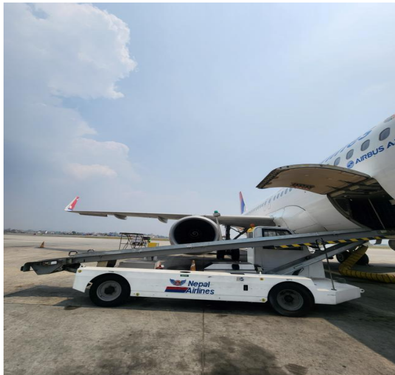
Figure B.6: Conveyor Belt
