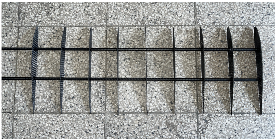
Figure A.4: Assembly of wing internal structure
