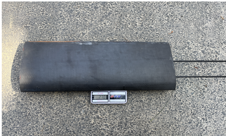
Figure A.8: Total Weight measurement of assembled wing
