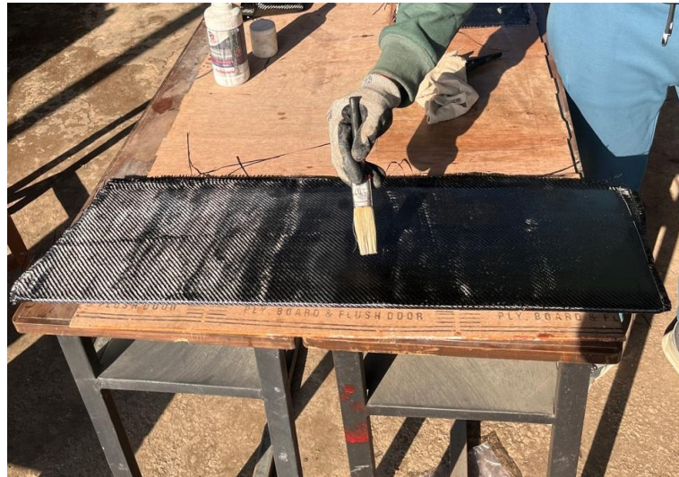
Figure A.1: Carbon Fiber layup process using wood mold
