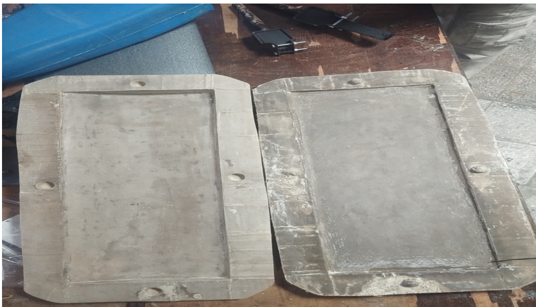
Figure 3.10: Two Part Molding
