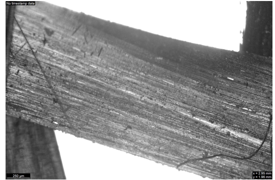
Figure 4.24: Smooth surface finish after resin curing
