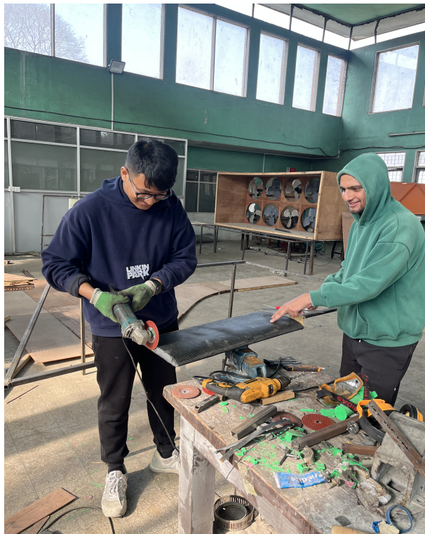
Figure A.6: Grinding off the surplus wing skin material.
