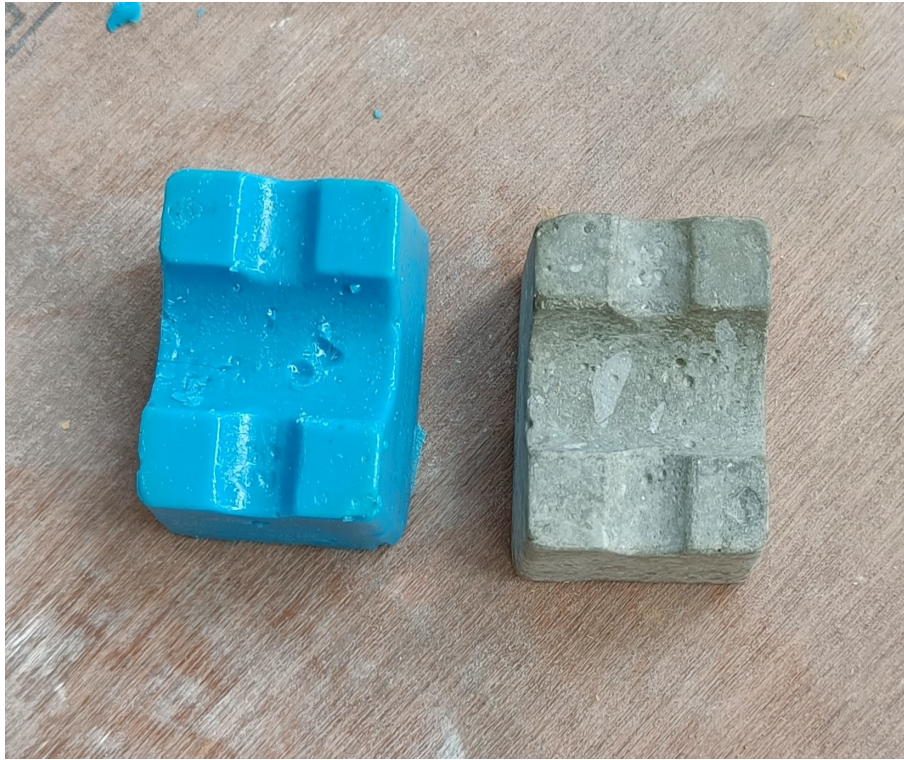
Figure 3.6: Mold generated from actual part
