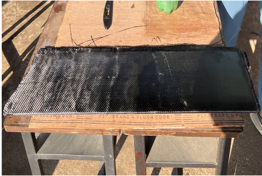
Figure 4.5: Carbon Fiber Wing Skin
