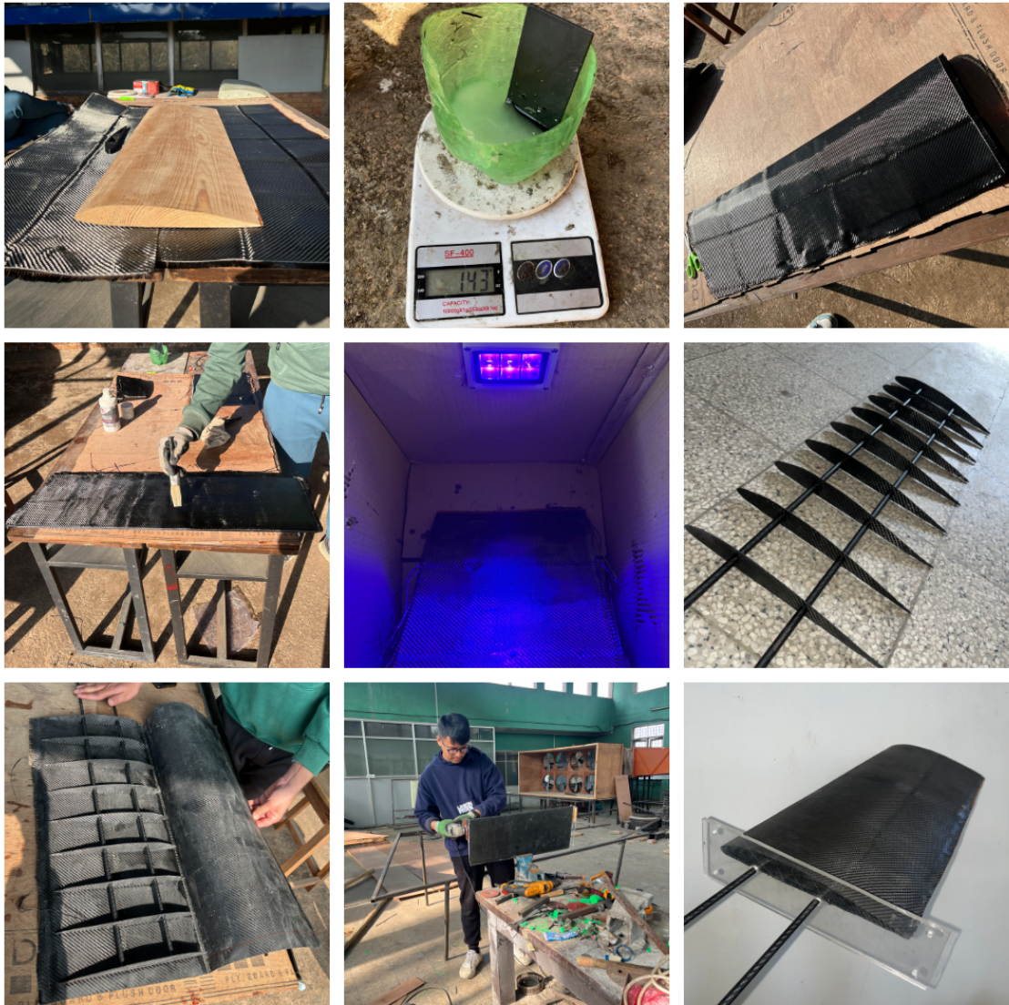
Figure 3.19: Process involved in fabrication of carbon fiber wing
