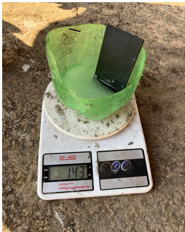
Figure A.2: Resin to Hardener mix weight measurement (100:40)
