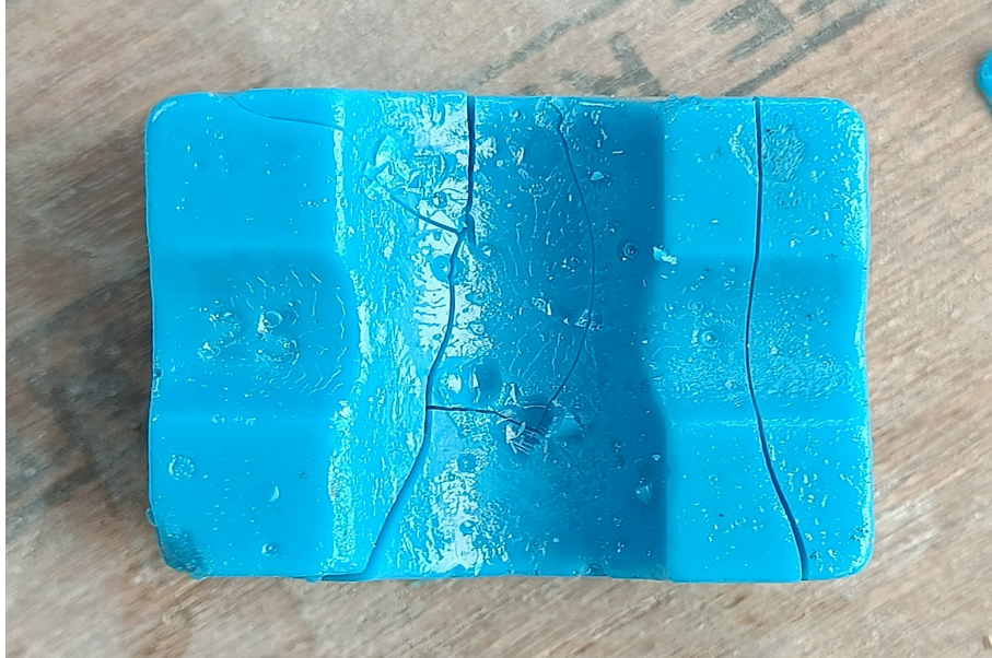
Figure 4.2: Silicon Mold Failure
