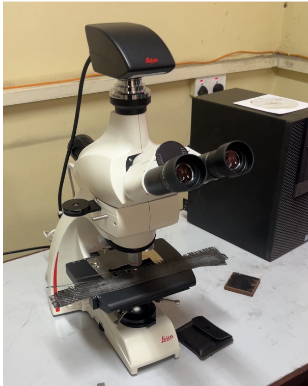
Figure B.1: Microscope setup for analyzing fiber diameter and resin-hardener distribution in the composite layup.
