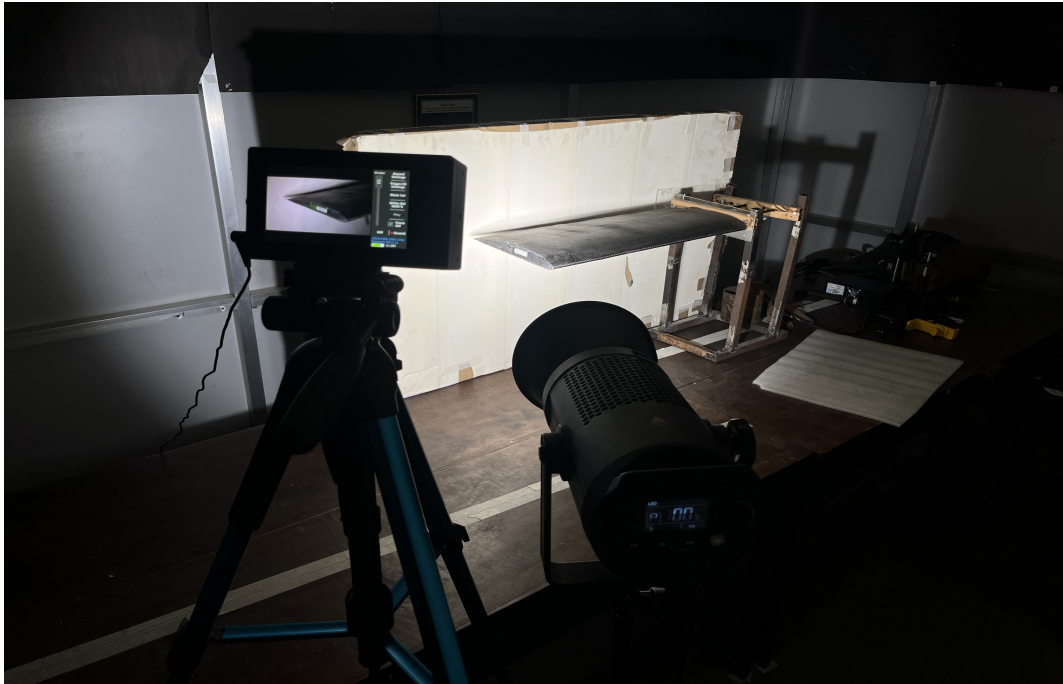
Figure 4.16: Experimental setup for capturing motion using high speed camera
