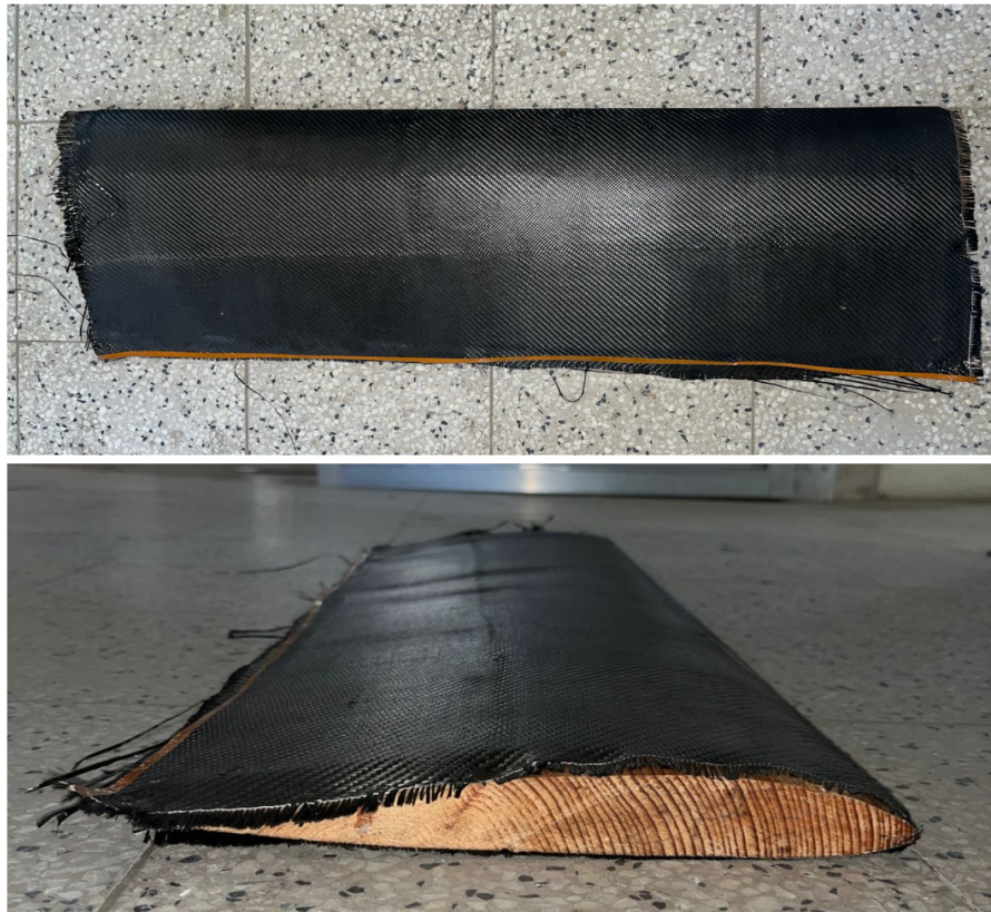
Figure A.3: Cured carbon fiber wing skin shaped using a wooden mold
