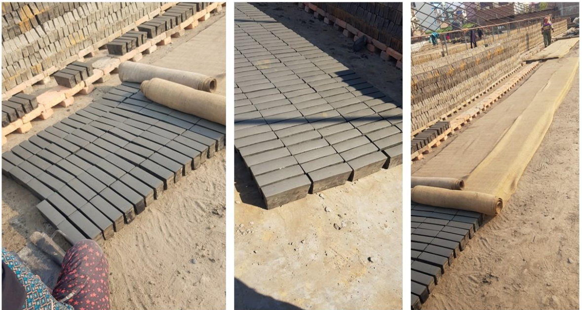
Figure 20. Making of raw Dachi brick
