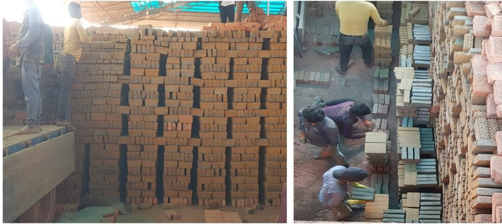
Figure 24. Sun dried brick stacked for burning
