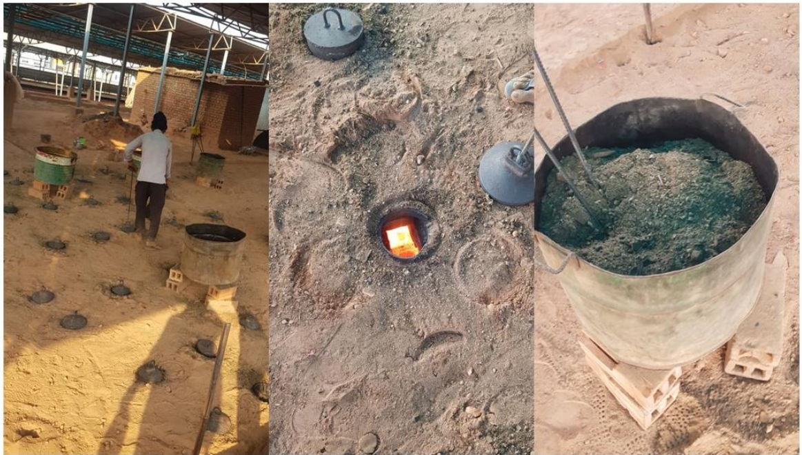
Figure 25. Brick burning inside kiln
