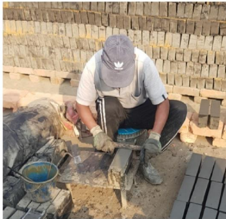
Figure 1: Fair face of brick is smoothed with a knife
