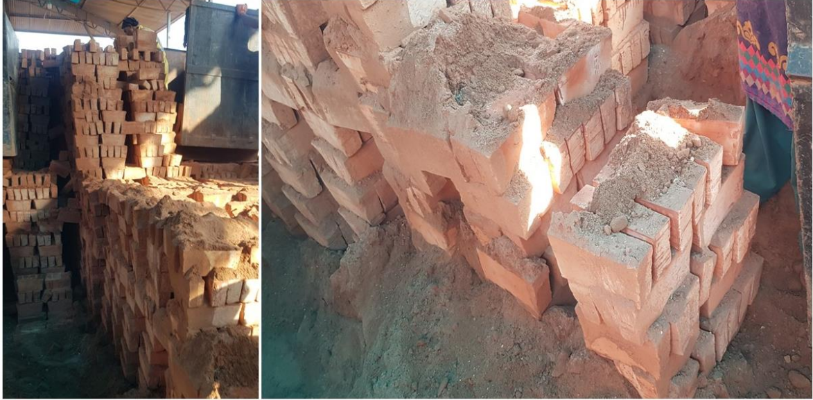
Figure 26. Taking out burnt brick from kiln
