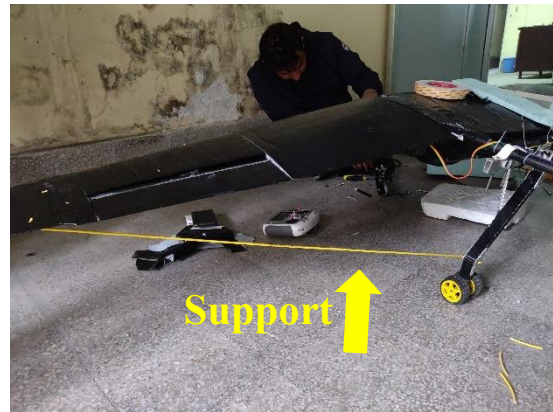
Figure 4-16 Addition of support to reduce the deflection
