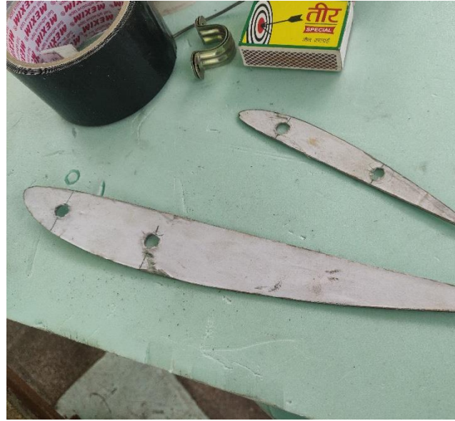
Figure 7-22 Steel ribs fabricated to visualize the wing offset from real design during manufacturing
