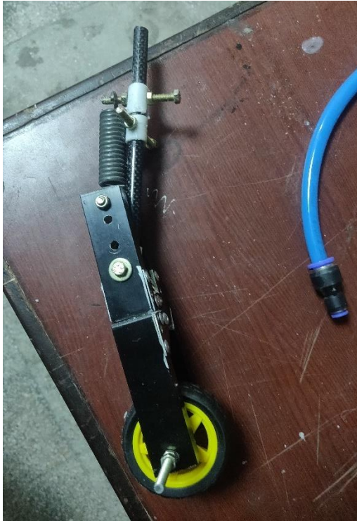
Figure 7-13 Final Design of rear landing gear with spring attachment for suspension
