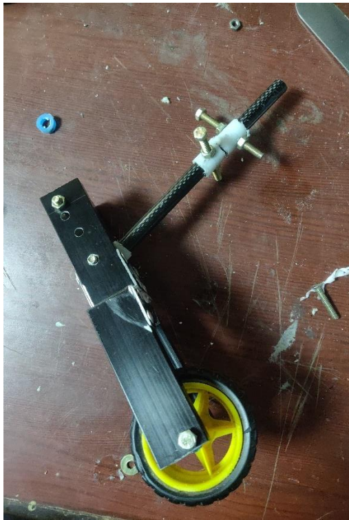
Figure 7-11 Final Design of rear landing gear (side view)
