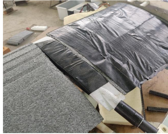
Figure 7-25 Wrinkled sections of wing as the foam did not support the stickiness of the duct tape
