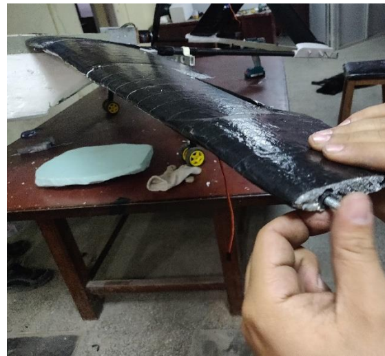
Figure 7-31 Stud fixation to wing
