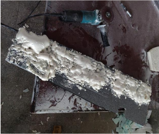
Figure 7-26 PU Foam sprayed wing section to obtain rigidity in spars
