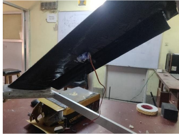
Figure 3-48: Servo motor mounted on tail wing
