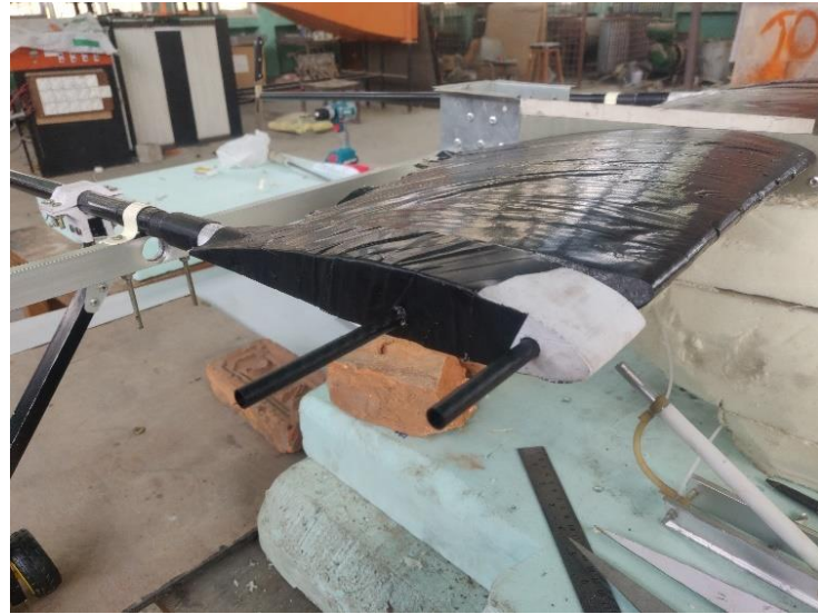
Figure 3-22: Spar connection in wing (twin spar)
