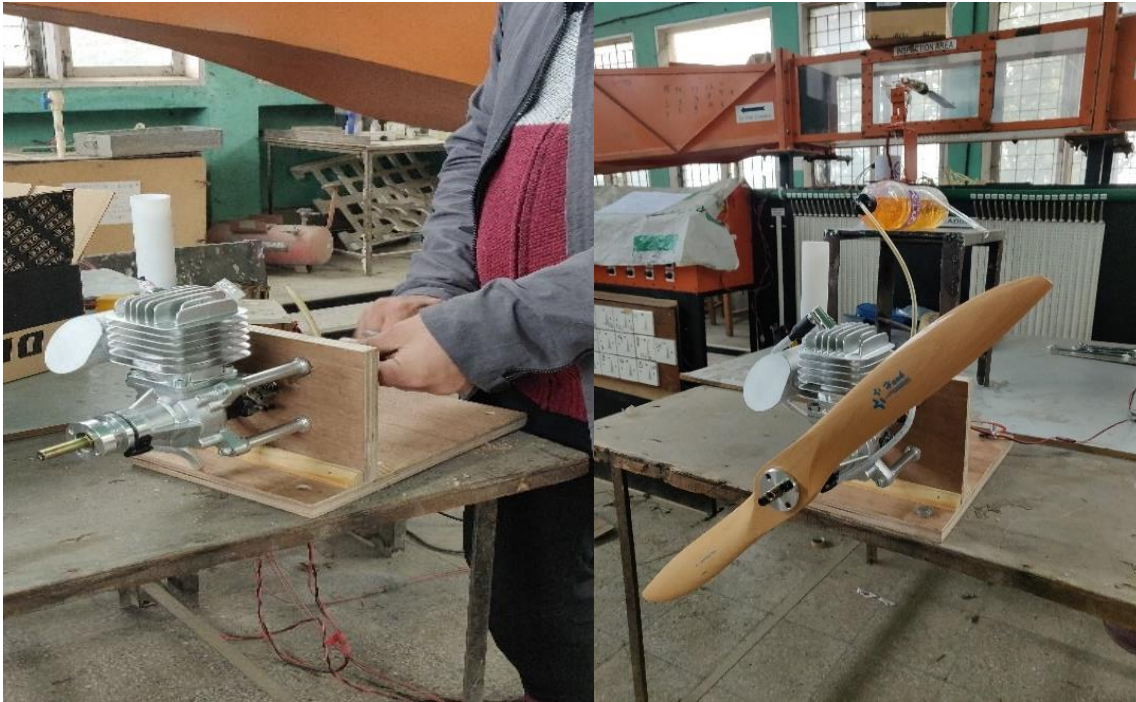
Figure 3-1: Piston Engine mounted on wooden frame
