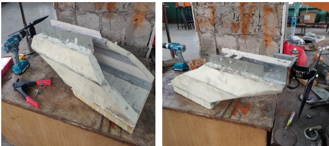
Figure 3-14: Fuselage (left side) sealed with PU Foam (on the left) and fuselage with motor propeller frame (on the right)
