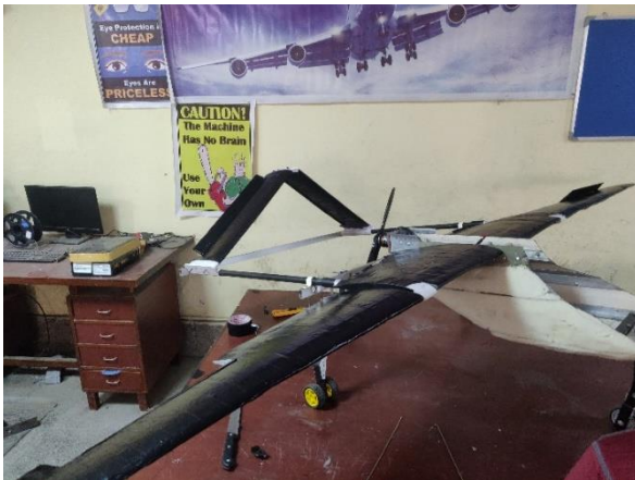
Figure 3-45: Surface smoothening using black tape and Fevicol
