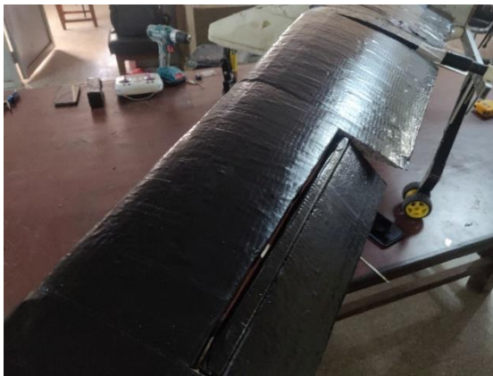
Figure 3-51: Aileron attached using 3 mm Carbon Fibre Rod
