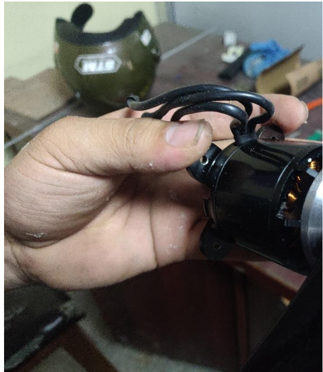
Figure 7-20 Newly fabricated motor and propeller clamp as original broke due to torsion
