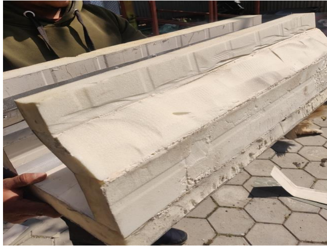
Figure 3-13: Initial development of fuselage using PU Foam Panel
