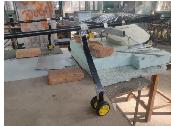
Figure 3-31: Side view of rear landing gear attached with 3D printed clamp
