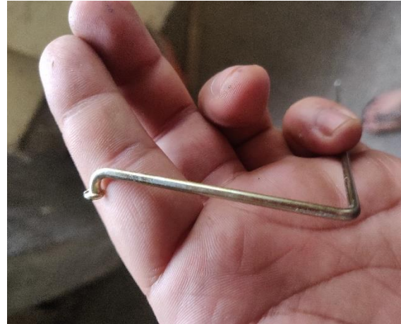
Figure 7-27 Links made out of bicycle spoke for servo linkage
