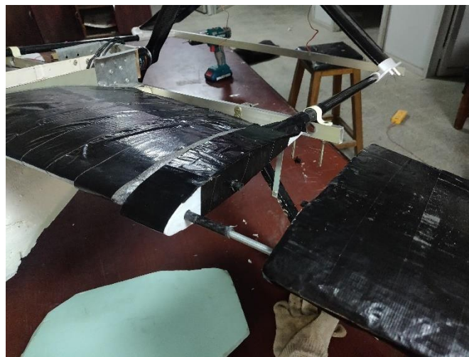
Figure 3-38: 6 mm stud fitted for wing end to end connection
