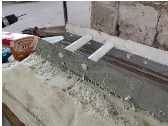
Figure 3-15: Nylon Bush attached in between wing sections for spar connection as well as rigidity
