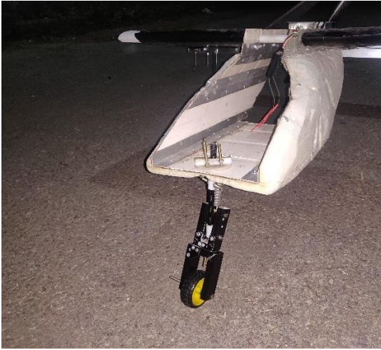
Figure 7-17 Landing gear backward position during ground testing
