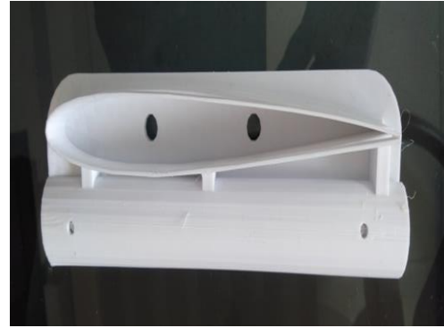
Figure 3-40: Wing attachment 3D printed adapter
