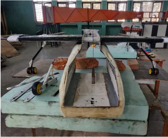
Figure 7-5 Fuselage front view during assembly
