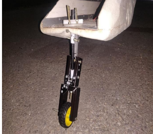
Figure 3-29: Nose landing gear into UAV
