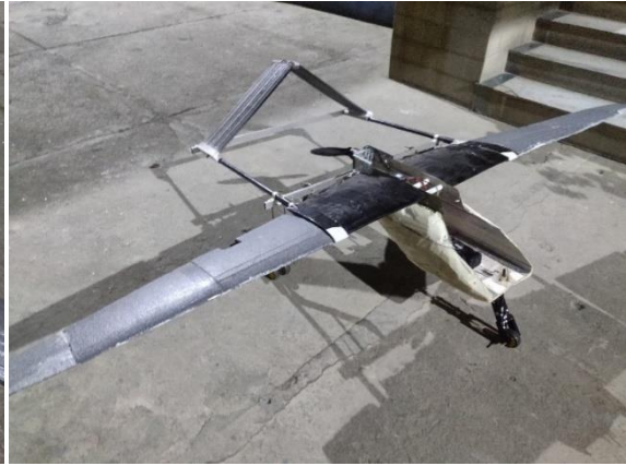
Figure 3-44: Ground testing of UAV with new design of Nose Landing Gear
