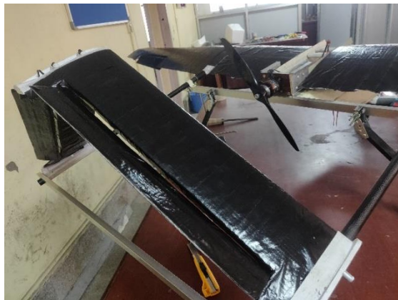
Figure 3-52: Stabilizers attached using 3 mm carbon fibre rod
