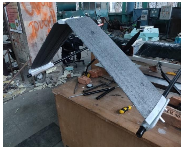
Figure 3-21: Tail connection without stabilizer cutting
