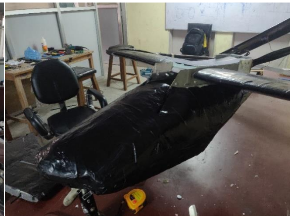
Figure 3-50: After wrapping the fuselage with black duct tape
