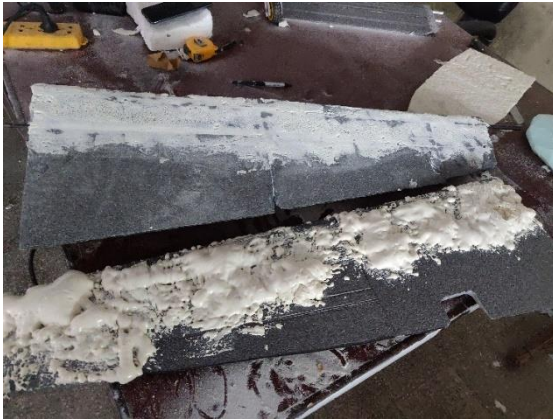
Figure 3-25: Wing section sprayed with PU foam and grinded to obtain the aerodynamic shape of the wing
