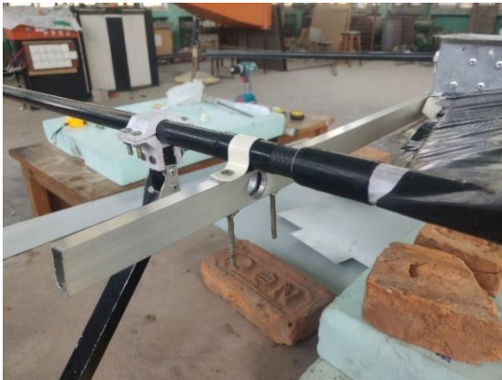
Figure 3-30: 3D printed clamps for rear landing gear attachment
