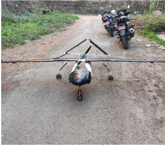
Figure 7-28 Ground testing of UAV before servo motor wiring
