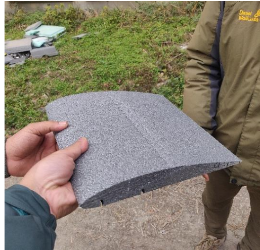
Figure 2-2: Sample wing section with spar fabricated by foam cutter
