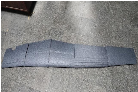
Figure 3-18: Wing sections as cut by CNC Foam Cutter
