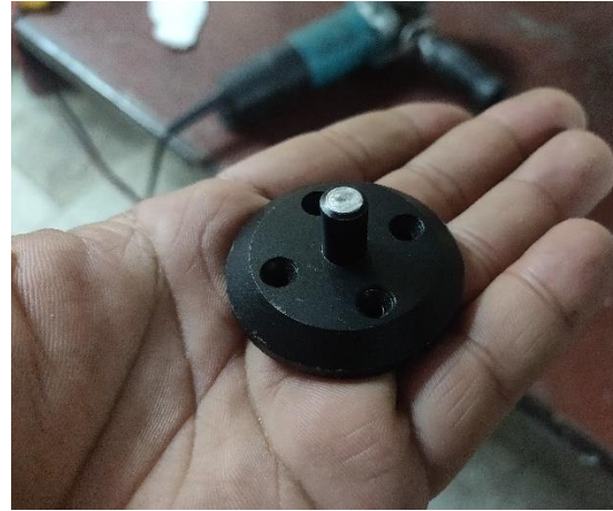
Figure 7-10 Failure of motor clamp due to high torsion during opening closing
