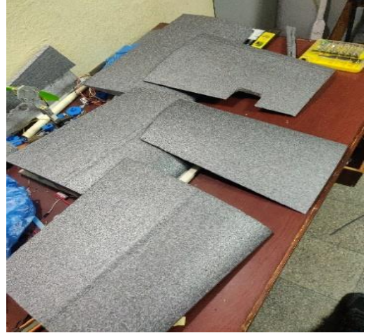
Figure 3-17: Airfoil profiles after cutting using foam cutter
