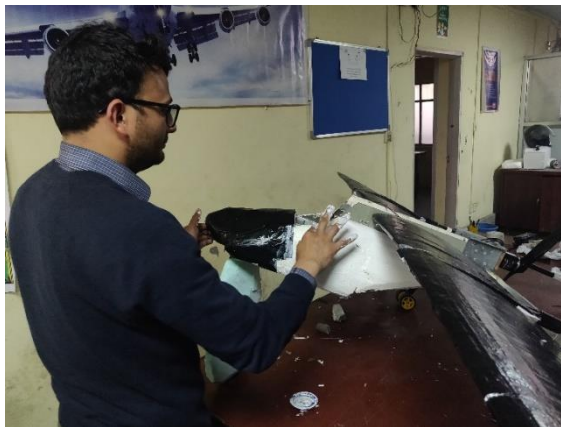
Figure 3-49: Fevicol sprayed over the fuselage PU foam body to increase stickiness with duct tape
