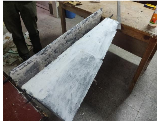
Figure 3-26: PU foam spread and grinded to wing for rigidity
