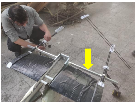
Figure 4-7 Rectangular bar addition behind the wing
