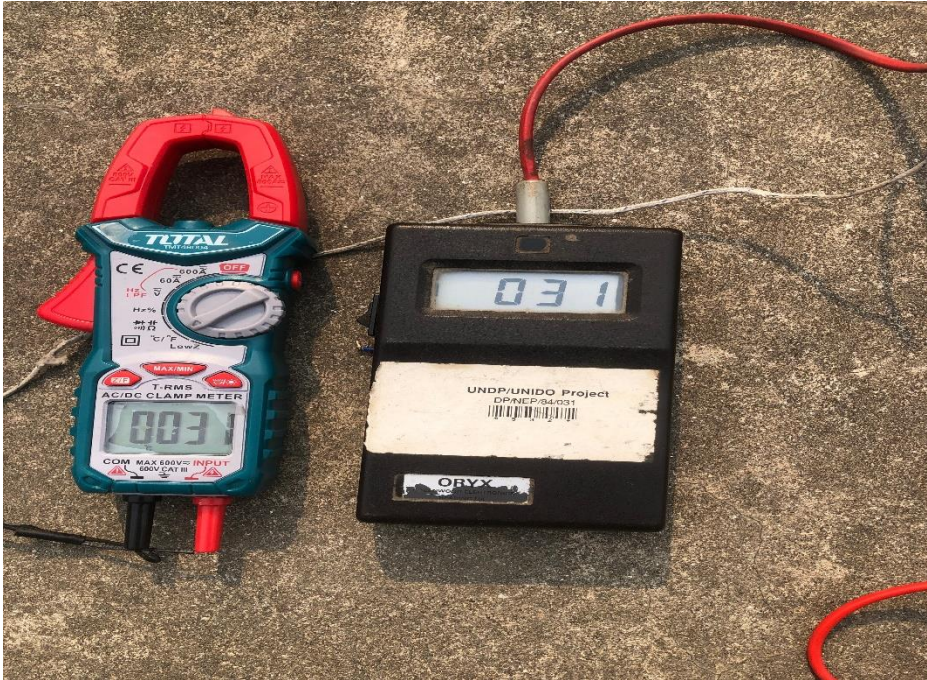
Photographs 1: Clampmeter and Oryx thermoCouple for Temperature Measurement
