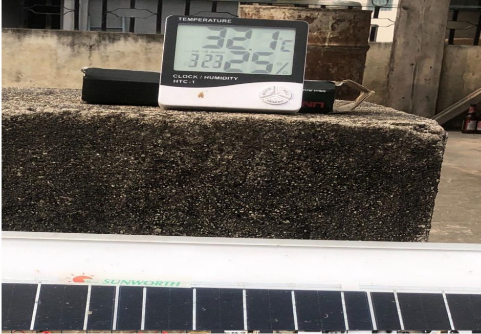
Photographs 3 : Digital Thermo hygrometer for measuring humidity
