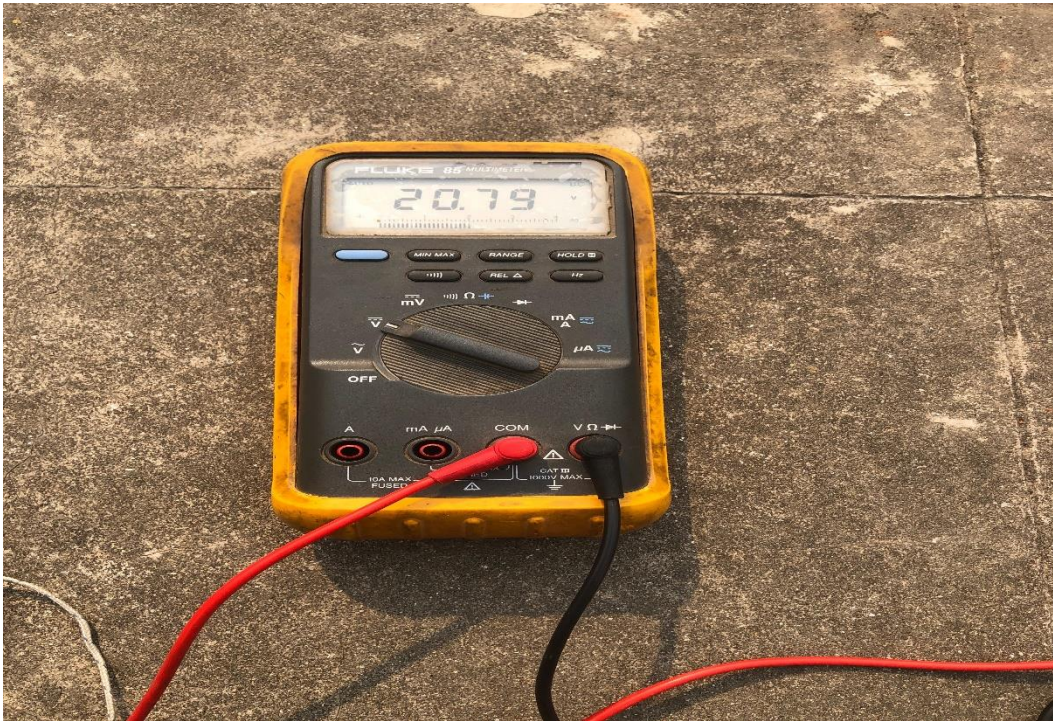
Photographs 2: Fluke Multimeter for measuring Current and Voltage
