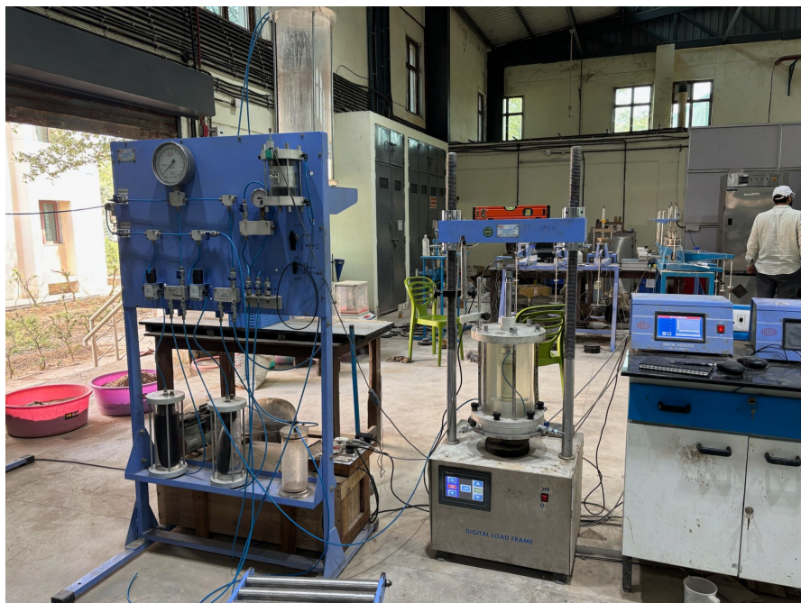
Figure B.13: Triaxial setup for UU test of sand sample.
