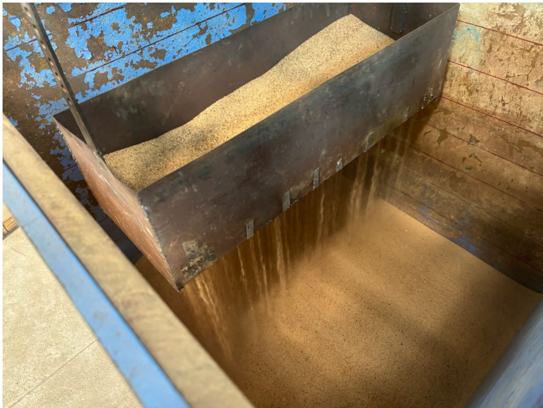
Figure 4.6: Pluviation method for sand deposition
