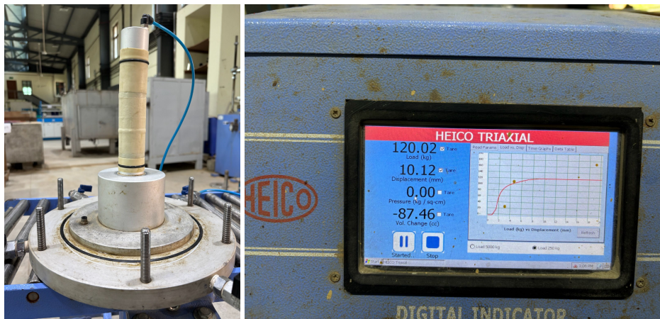
Figure B.12: Sample preparation for triaxial testing and tested sample.
