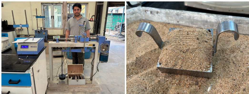
Figure B.9: Direct shear test of sand.
