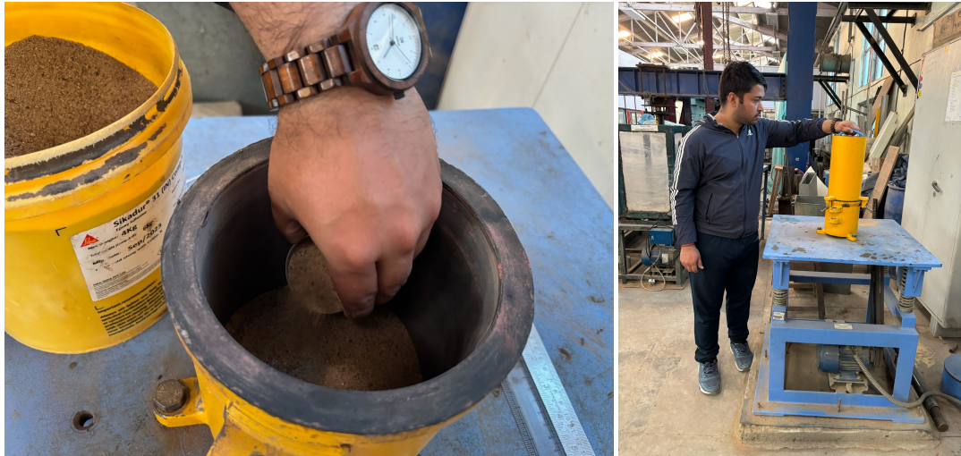
Figure B.8: Relative density test of sand.
