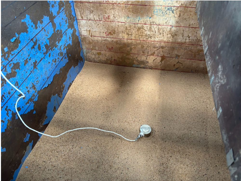
Figure B.14: Leveling of sand bed and installation of pressure cell.
