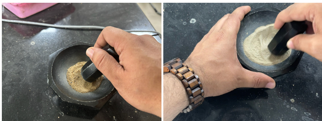
Figure B.10: Sample preparation for XRD analysis.
