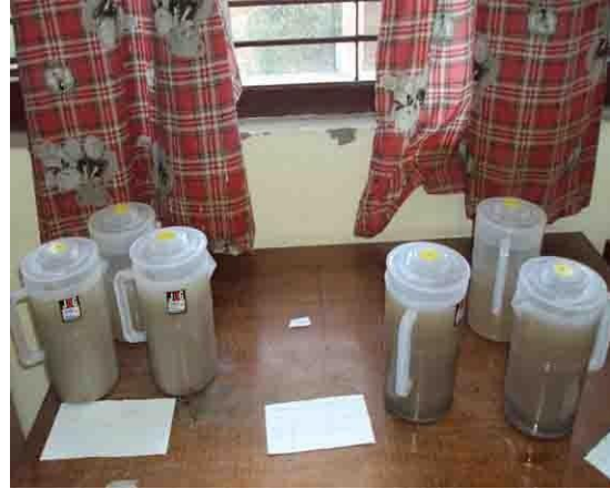
Figure 5: Crushed samples placed in jugs for settlement
