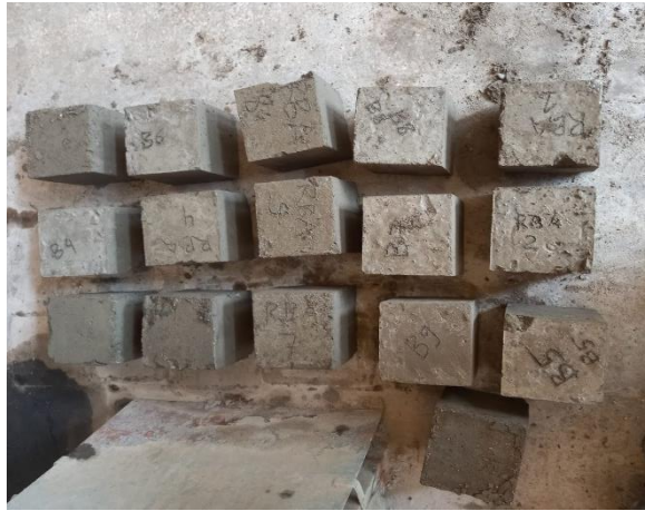
Figure 36: De-molding of cubes after 24 hours
