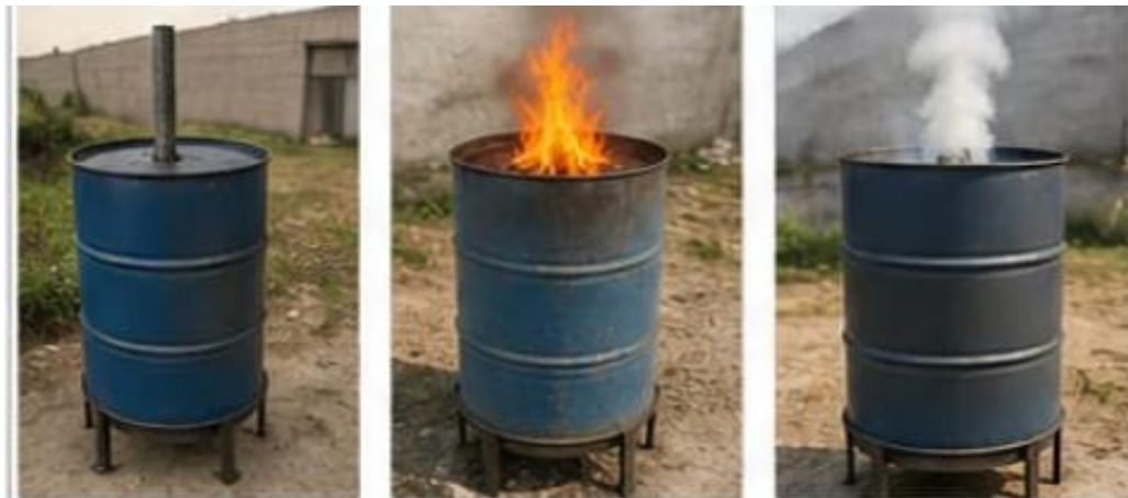
Figure 10: Pyrolysis process (Ignition from bottom of drum)
