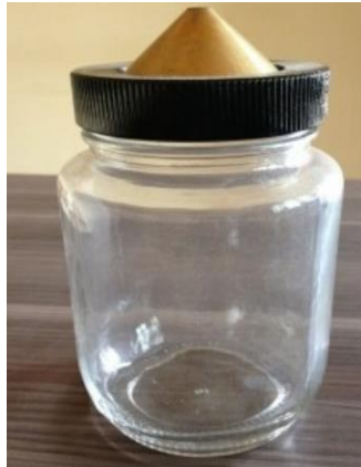
Figure 14: Pycnometer (Specific gravity test for fine aggregate)
