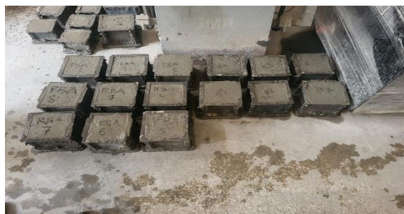
Figure 34: Mold Cubes (150 mm × 150 mm × 150 mm)
