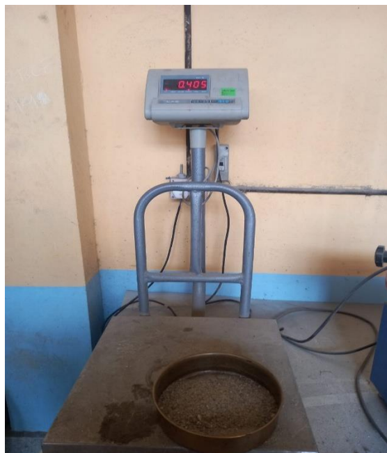
Figure 44: Fine aggregate for sieve analysis (weighing: 300g):
