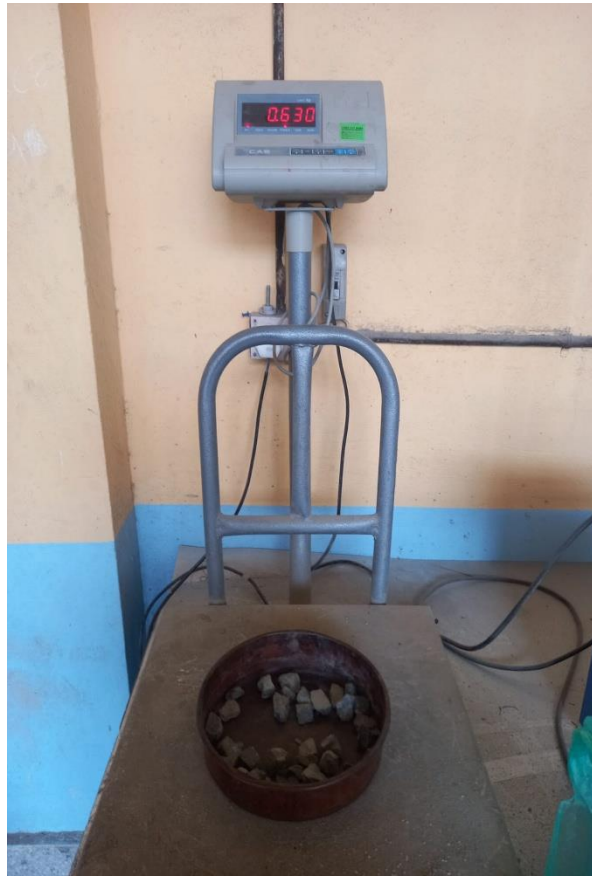
Figure 45: coarse aggregate for sieve analysis (weighing: 300g)
