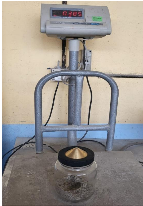
Figure 49: sand and pycnometer weighing
