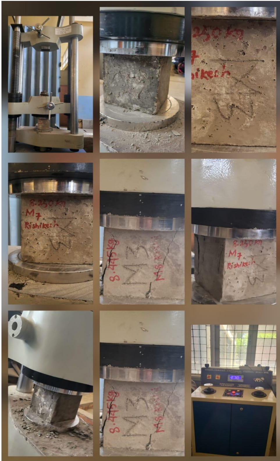
Figure 42: After cube specimen keep under UTM: failure pattern
