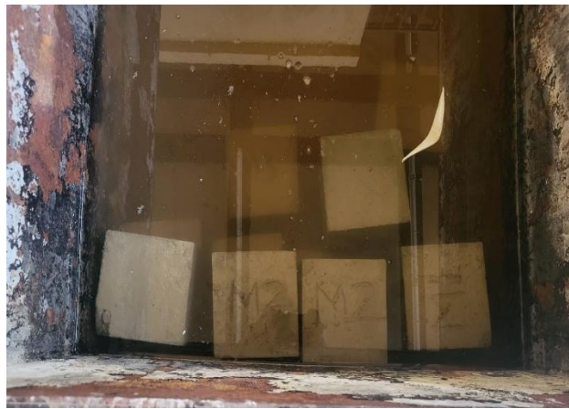
Figure 37: Curing of concrete for curing period of 7, 14 and 28 days
