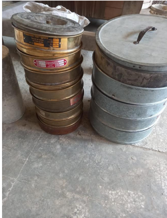
Figure 43: Sieve Sizes set up for fine and coarse aggregate
