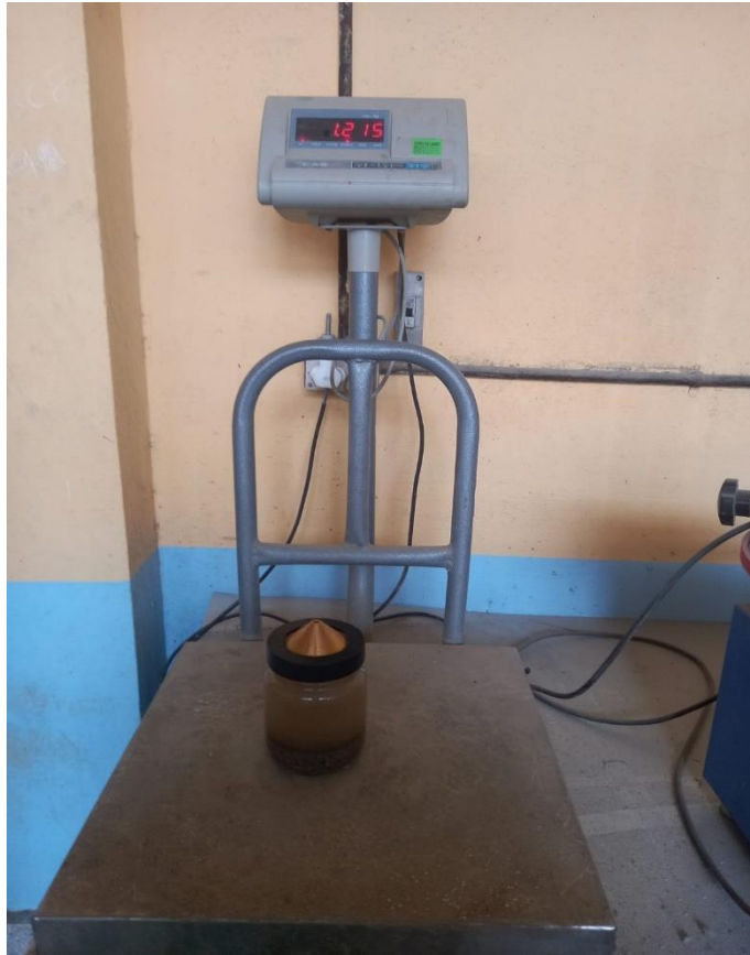
Figure 47 sample with water and pycnometer weighing
