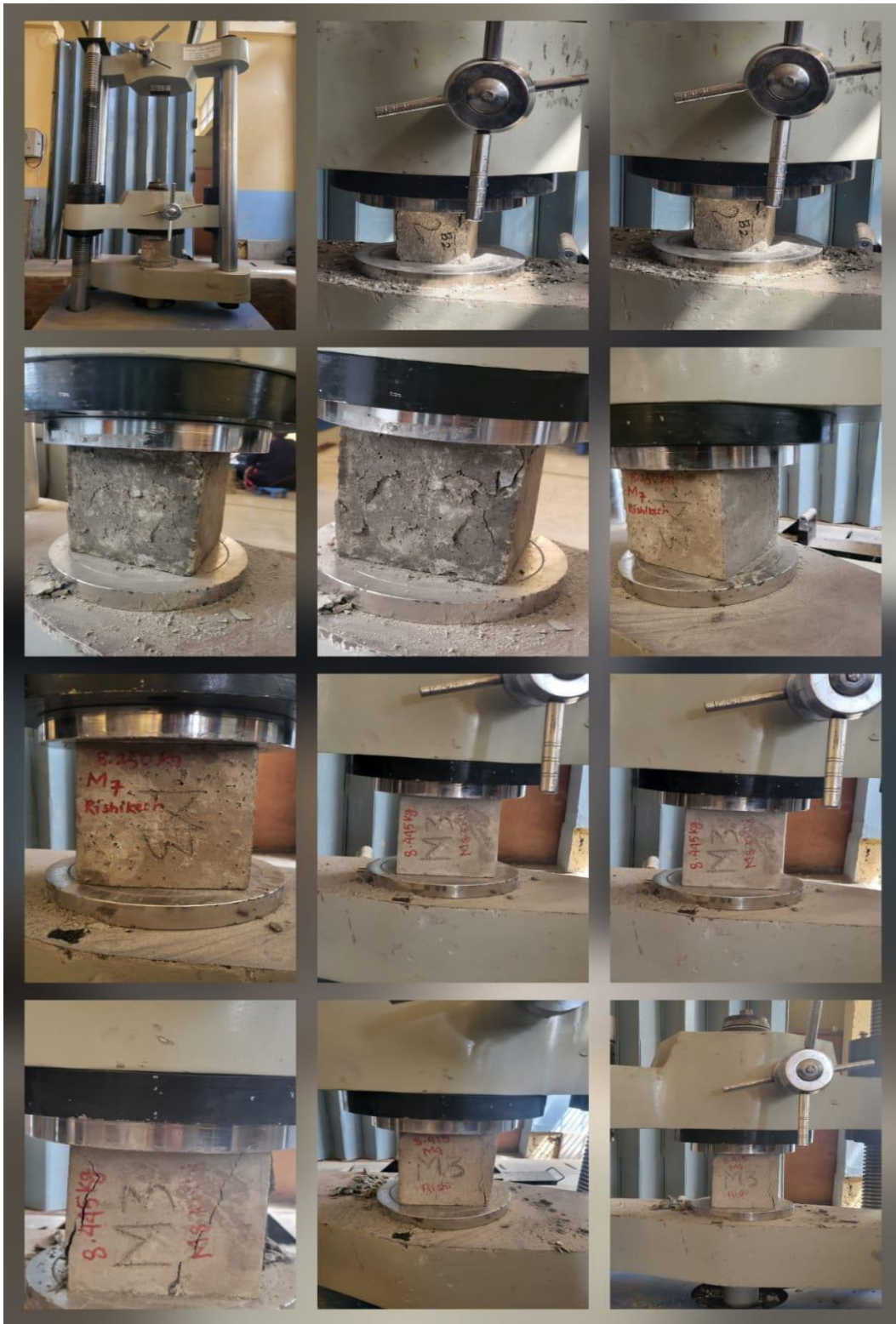
Figure 41: Testing of cube specimens for 7, 14 and 28 days
