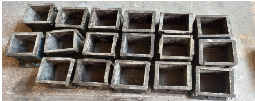
Figure 34: Mold Cubes (150 mm × 150 mm × 150 mm)
