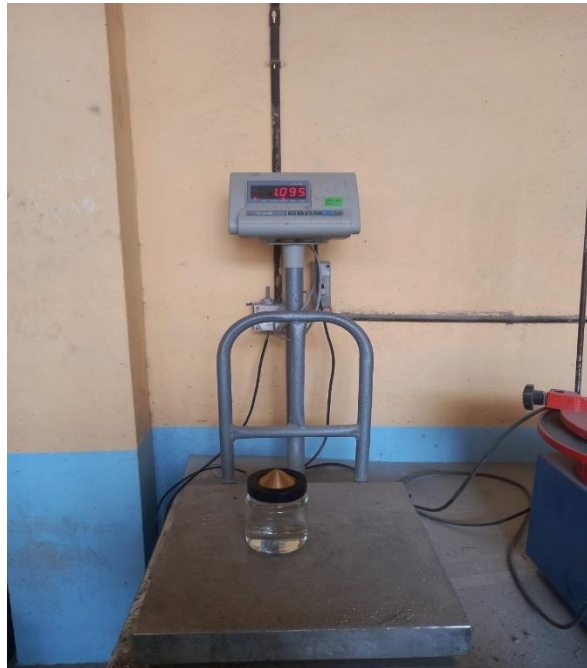
Figure 48 : water and pycnometer weighing
