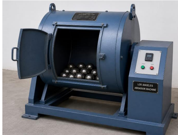
Figure 13: Los Angeles' machine test (coarse aggregate)
