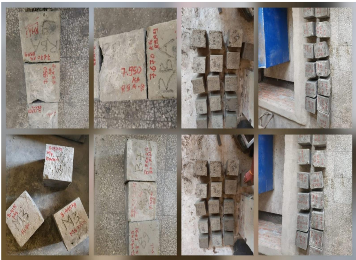
Figure 40: Cube specimens ready for testing in UTM
