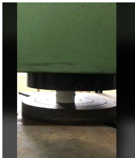
Figure 3.8: Compression Testing in UTM
