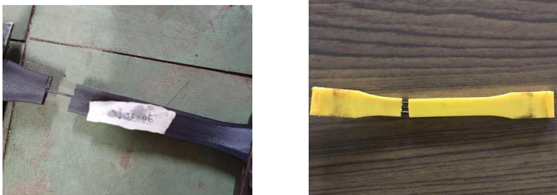
Figure 4.2: Tensile test result of wire-reinforced
