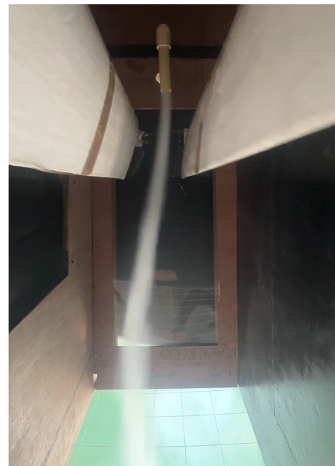
Figure 4.52: Gust Profile ( 3Hz , 200mm spacing, 10^\circ , 200mm chord)
