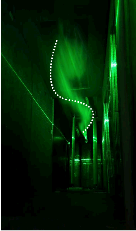
Figure 4.45: Gust Being Developed (4 Hz , 300 mm spacing, 15°, 250 mm chord) at t = 5.63 s
