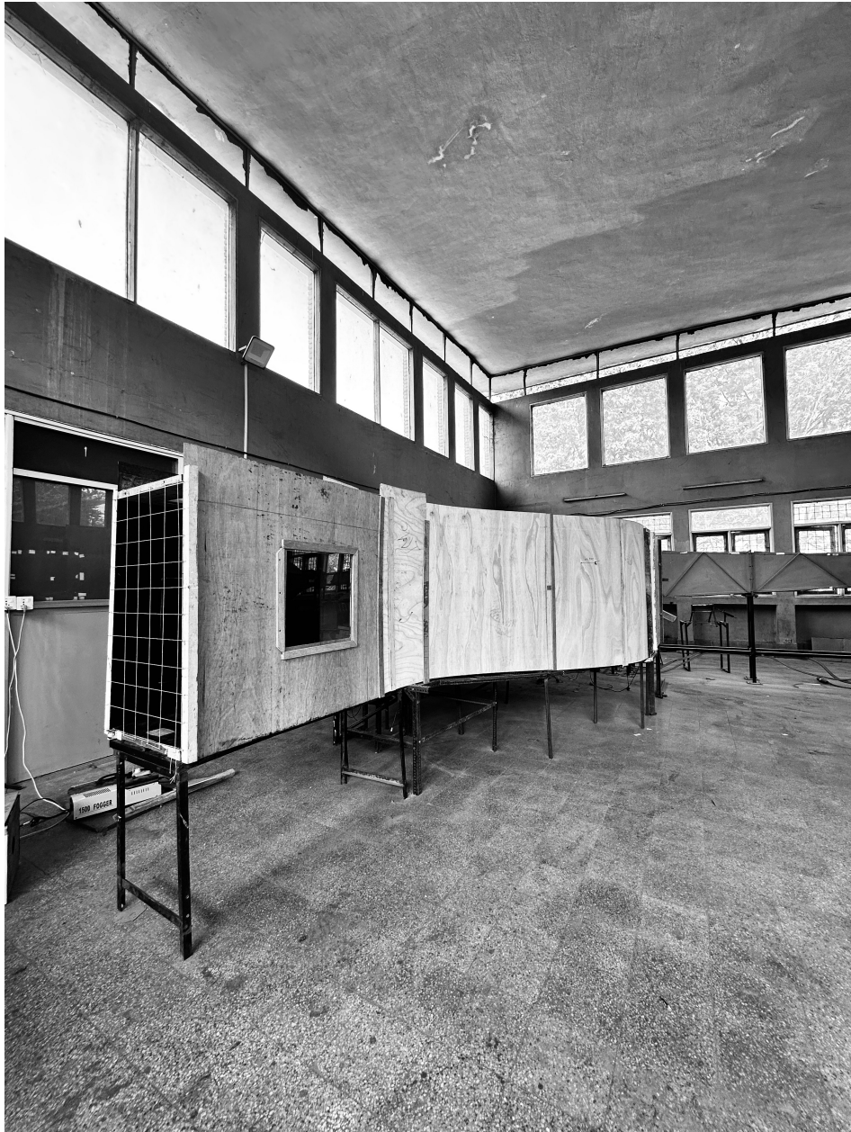
Figure C.12: Fabricated Wind Tunnel
