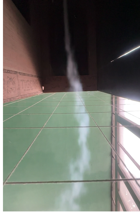
Figure 4.54: Gust Profile ( 4\text{ Hz} , 300\text{ mm} spacing, 15^\circ , 200\text{ mm} chord)
