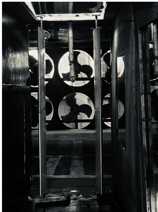
Figure 3.23: Integration of Vanes in the Wind Tunnel
