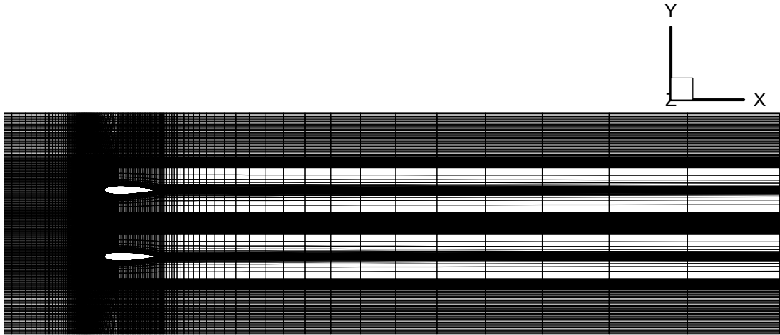
Figure 3.8: Coarse Mesh Domain for 25 cm chord
