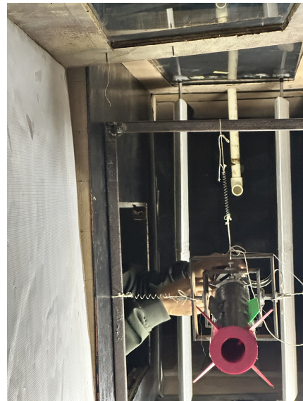
Figure C.16: Rocket Integration in Wind Tunnel with Gust Generator
