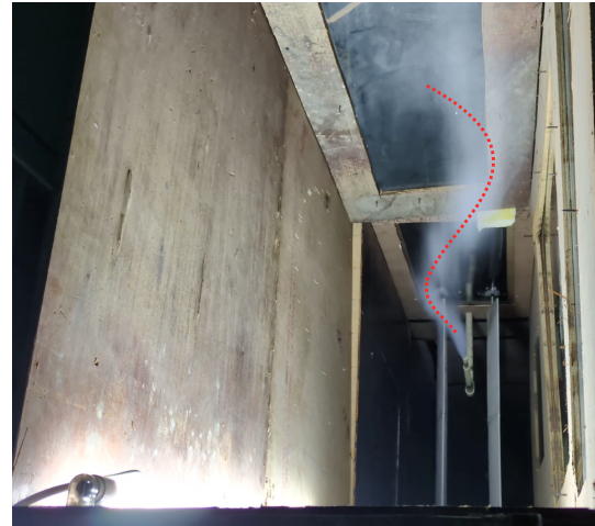
Figure 4.50: Gust Profile ( 4Hz , 200mm spacing, 15^\circ , 250mm chord) at t = 21.65s
