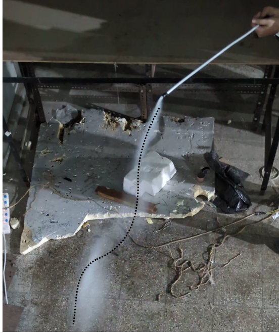
Figure 4.34: Smoke Visualization for Observing Flow Uniformity at Outlet of the wind tunnel
