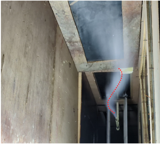
Figure 4.49: Gust Profile ( 4Hz , 200mm spacing, 15^\circ , 250mm chord) at t = 21.62s
