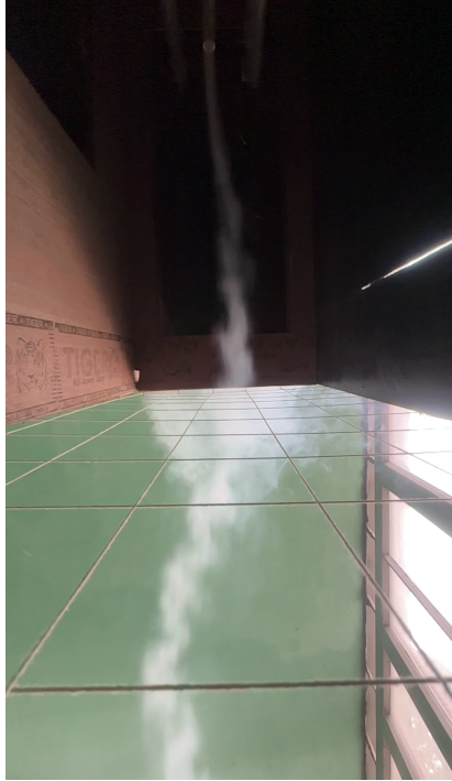
Figure 4.53: Gust Profile ( 4\text{ Hz} , 200\text{ mm} spacing, 15^\circ , 200\text{ mm} chord)
