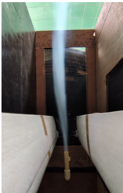
Figure 4.51: Gust Profile ( 2Hz , 200mm spacing, 10^\circ , 200mm chord)
