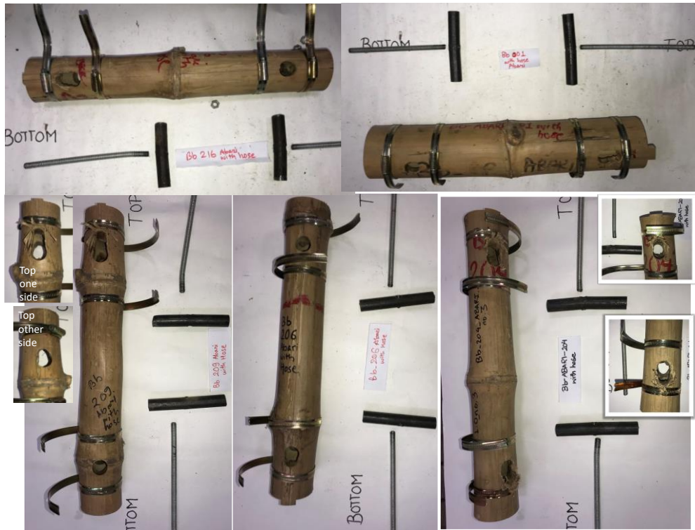
Figure 4.28 B. balcooa Shaft-bolt connection with hose clamp
