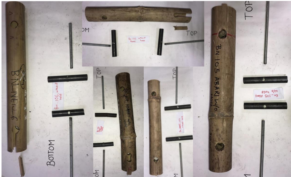
Figure 4.31 B. nutans Shaft-bolt connection without hose clamp
