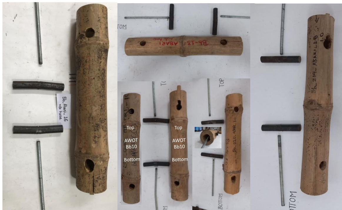
Figure 4.29 B. balcooa shaft-bolt connection without hoseclamp
