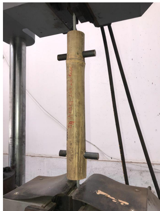
Figure 3.14 Shaft-bolt connection bring tested in the UTM
