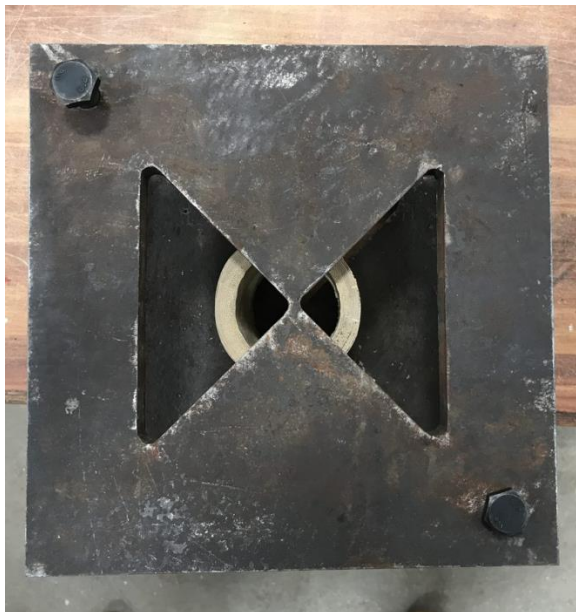
Figure 3.12 A Shear Test Setup using shear apparatus
