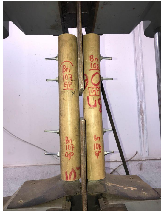
Figure 3.13 Gusset-plate connection bring tested in the UTM
