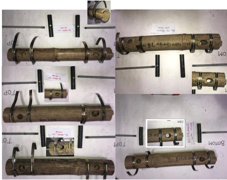
Figure 4.30 B. nutans Shaft-bolt connection with hose clamp
