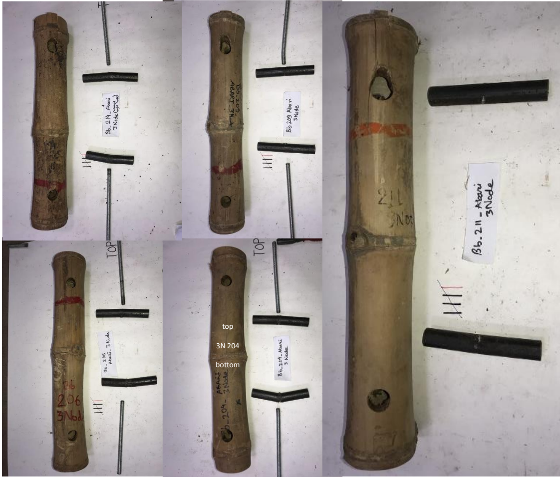
Figure 4.32 B. balcooa Shaft-bolt connections (Noded near bores)
