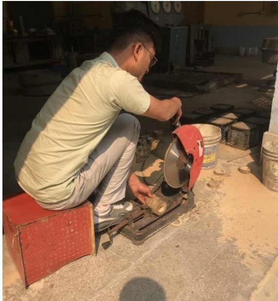
Figure 3.11 A bamboo specimen being prepared for testing. The picture shows a bamboo culm being cut into a smaller section of uniform length and diameter using a saw
