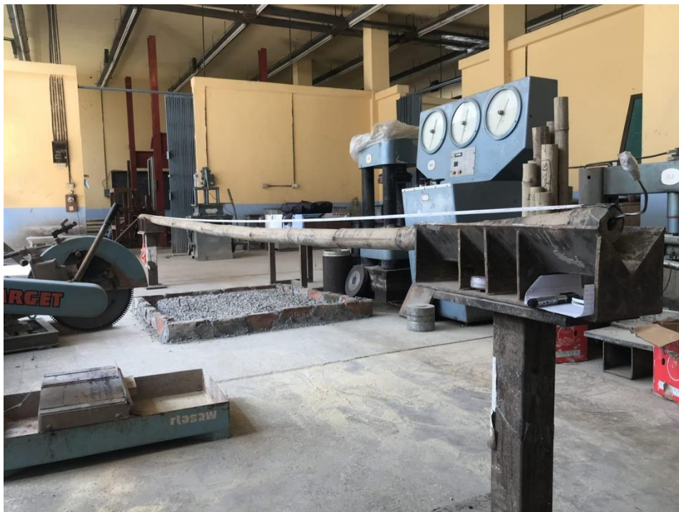
Figure 3.10 Setup for measuring geometric data of bamboo culms
