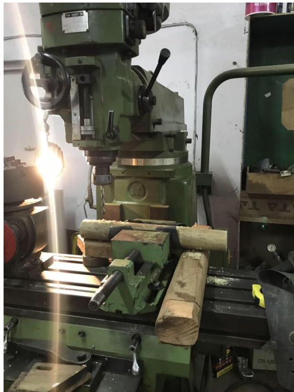
Figure 3.16 Connection Specimen Fabrication using Milling Machine
