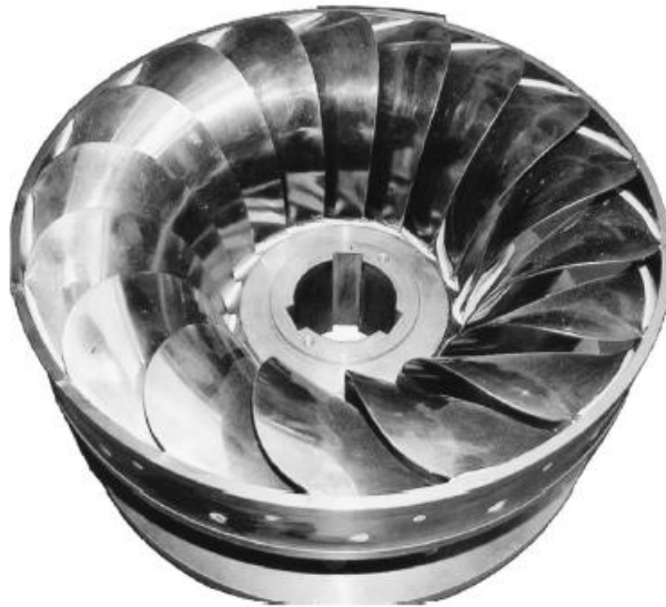
Figure 2.1: Runner of small Francis turbine
