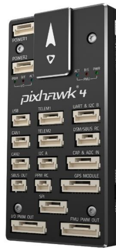
Figure A.8: Pixhawk 4® Controller
