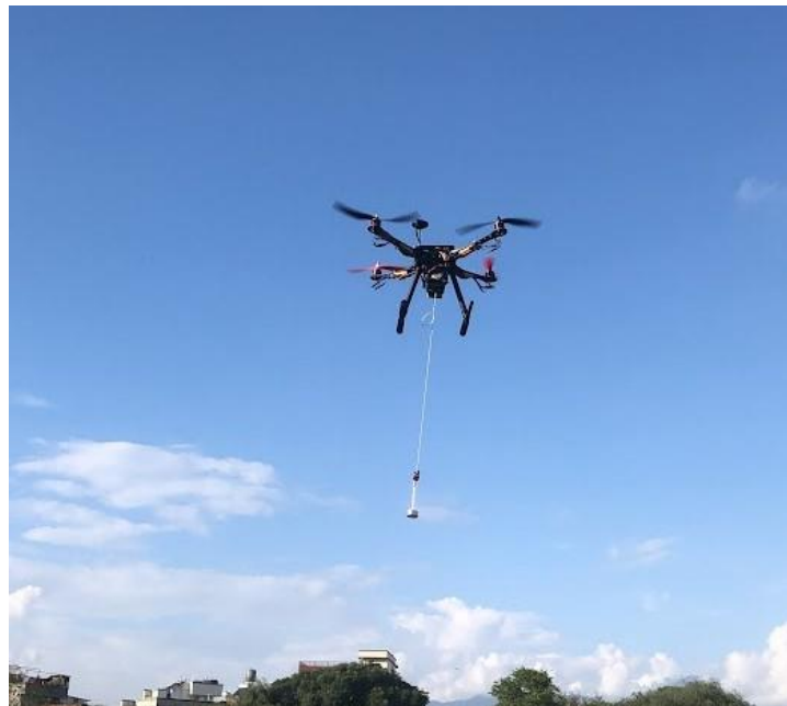
Figure 4.3: Quadrotor with 0.1 kg payload
