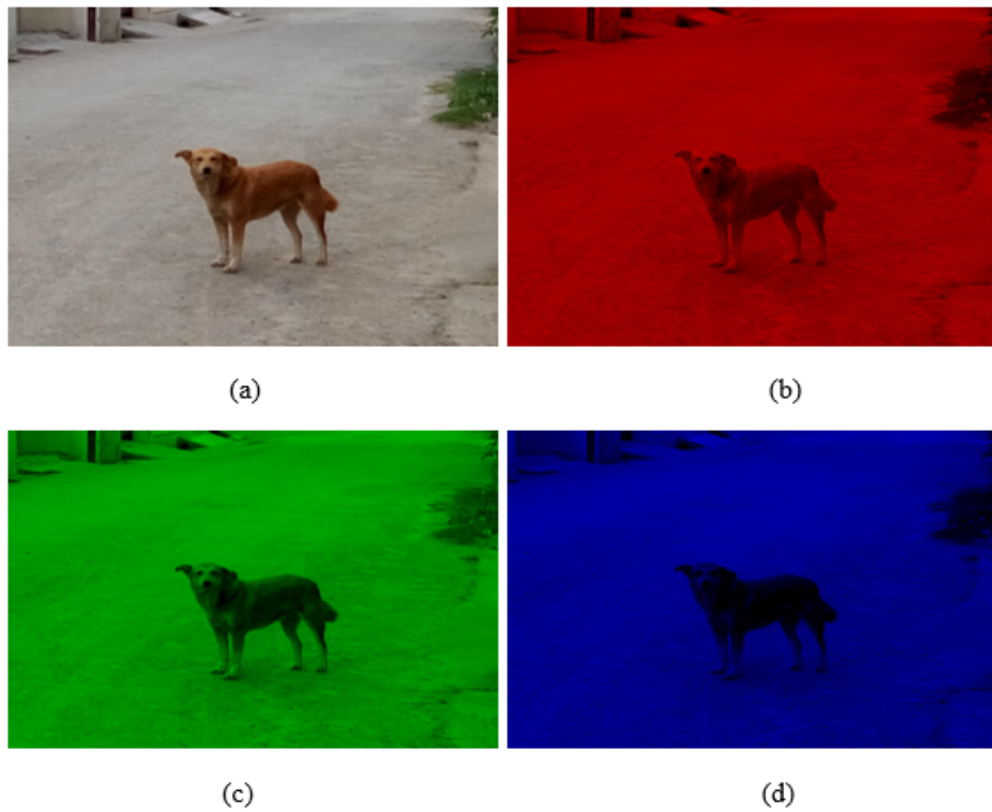
Figure 3.4: Original image and Red, Green and Blue component of an image. (a) Original image. (b) Red component. (c) Green component. (d) Blue component.
