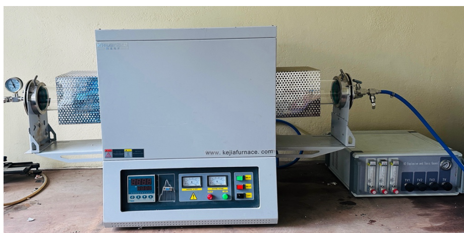
Figure 5. Heat annealing in Tube Furnace with Nitrogen atmosphere
