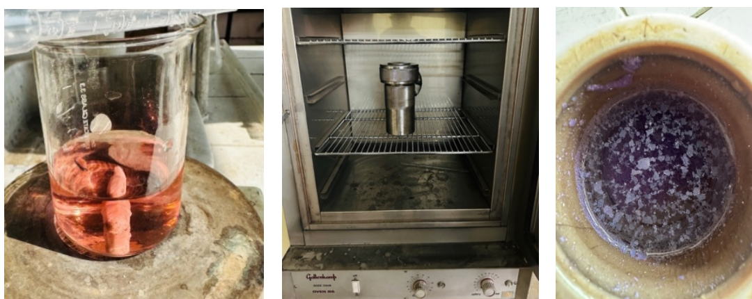
Figure 4. Precursor solution preparation, Hydrothermal synthesis and ZnCo LDH
