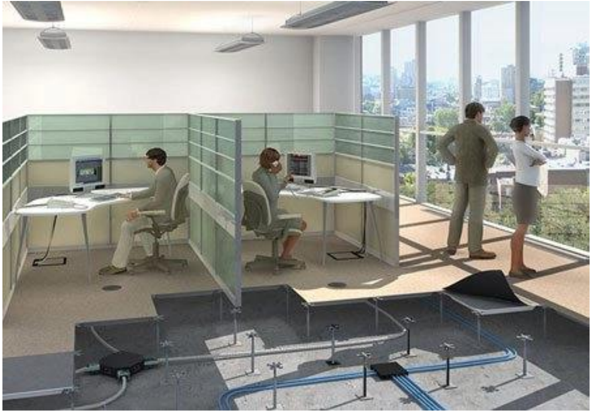
Figure 9: Underfloor Air Ventilation
