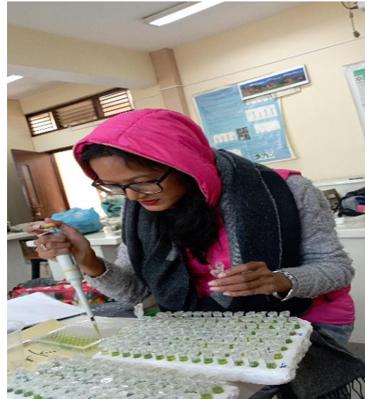
Photos of weighing and filling microplate using micropipette
