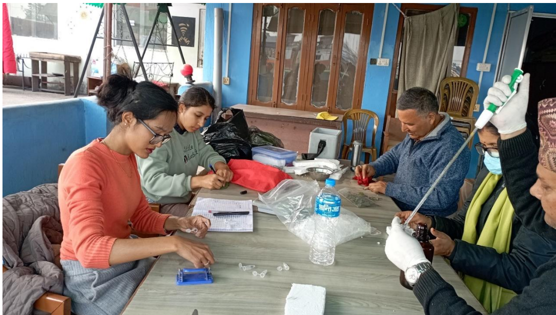
Photos of using DMSO 4 Solvent and eppendorf tube for chlorophyll extraction
