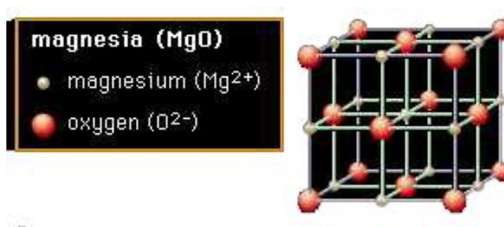
Figure 7: MgO crystal structure 15
