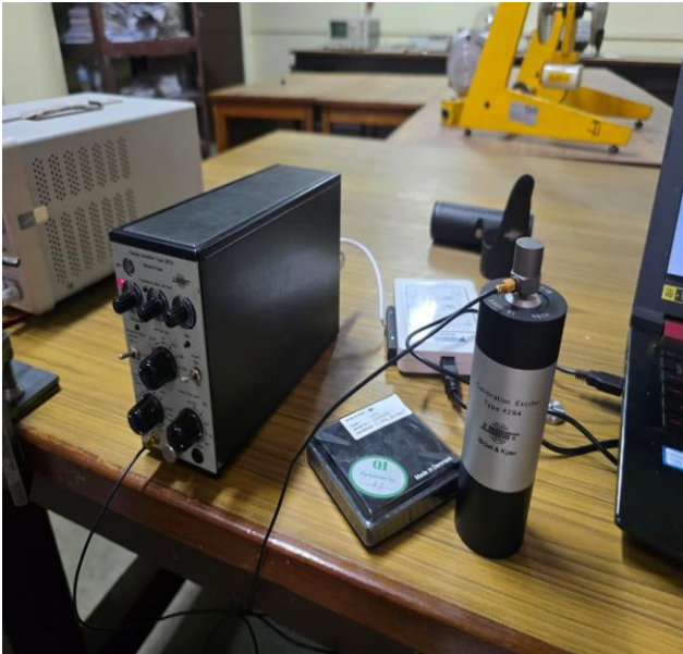
Figure 5: Accelerometer Calibration using Calibrator
