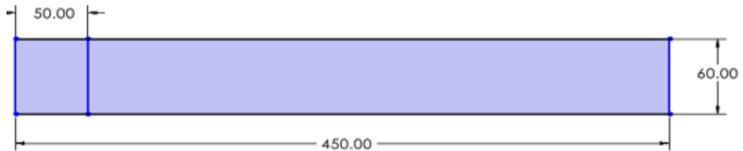
Figure 4.2: Dimensions of normal cantilever beam from top view
