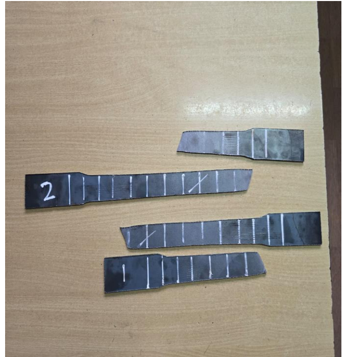
Figure 2: Test Specimen after Tensile Testing
