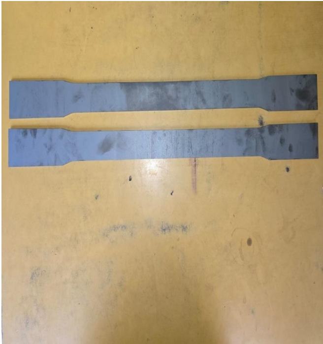
Figure 1: Test specimen for Tensile Testing
