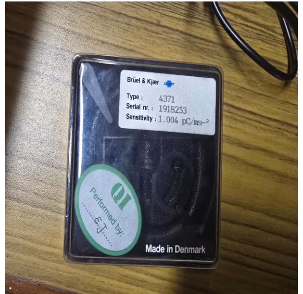
Figure 6: Accelerometer with its sensitivity
