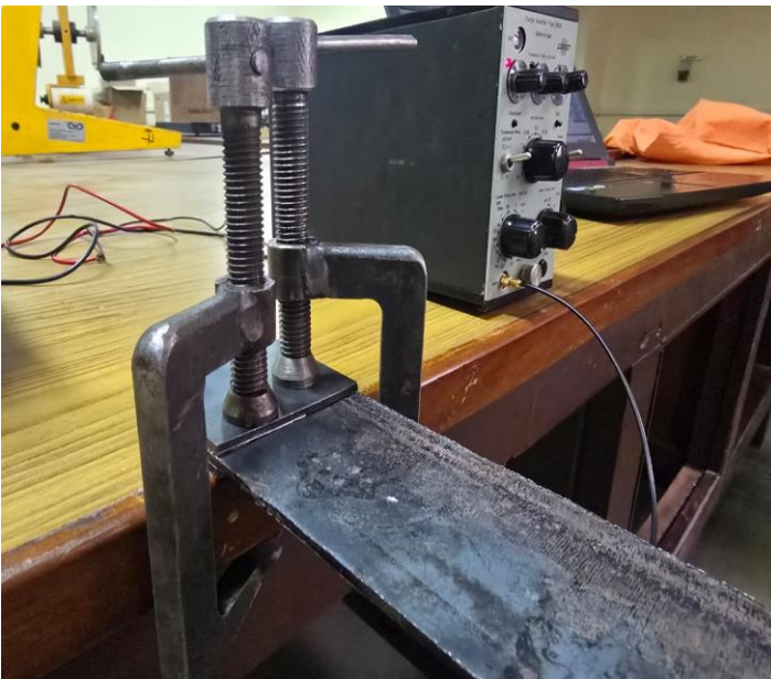
Figure 11: Applying Boundary Conditions to the specimen
