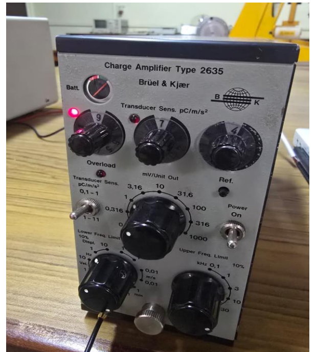
Figure 8: Charge Amplifier after adjusting the Sensitivity
