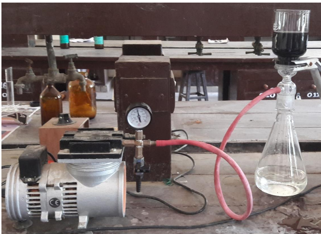
Fig. 4.2 (c) Purification of oxidized MWCNTs by Suction pump
