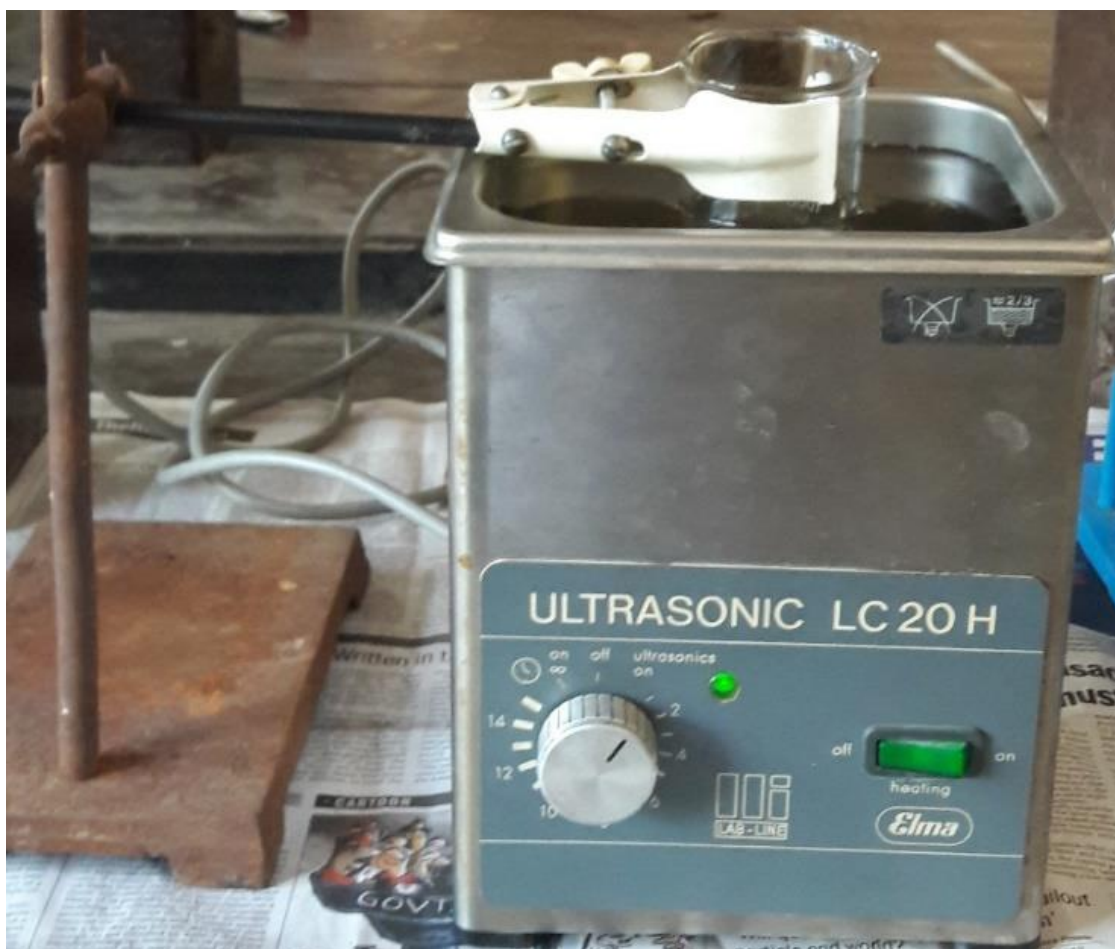
Fig. 4.2 (e) The process of stirring the solution by sonication
