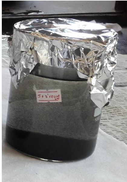
Fig. 4.4 (a) Well dispersed oxidized MWCNTs solution
