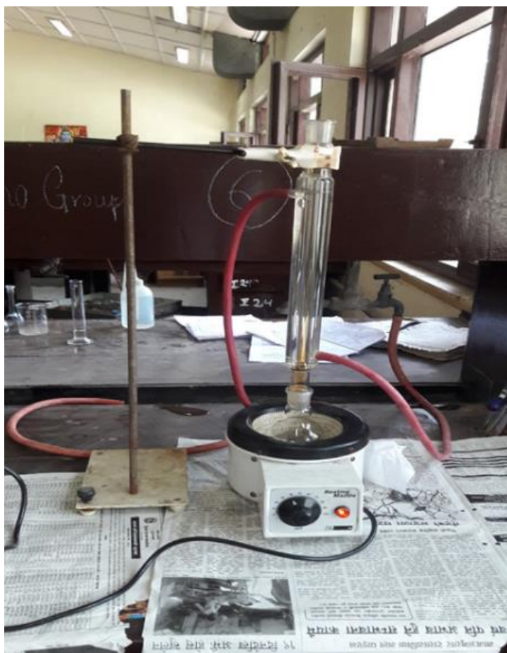
Fig. 4.2 (a) Oxidation of MWCNTs by acid reflux method
