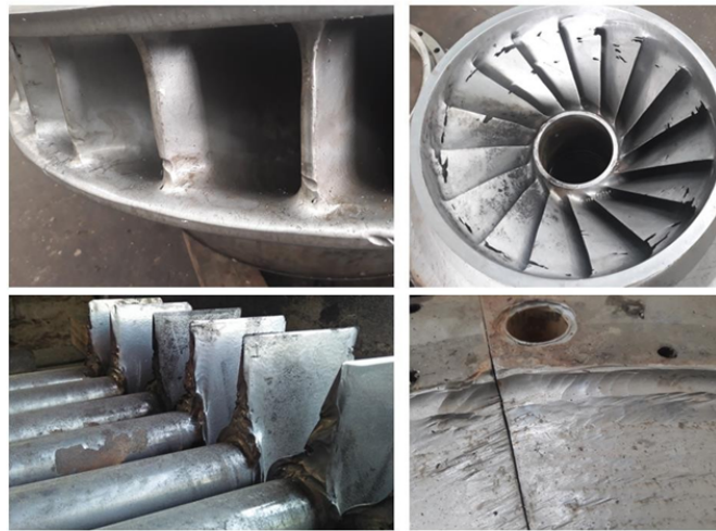
Figure 5.15: Erosion in the runner and guide vanes of the plant
