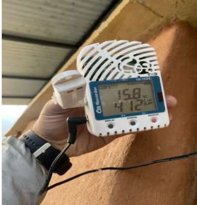
Figure 9 Co2 recorder used to collect outside temperature at Dekaido Onseen
