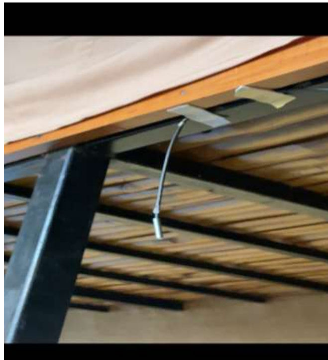
Figure 10 Hobo Data logger used to collect indoor temperature at Dekaido Onseen
