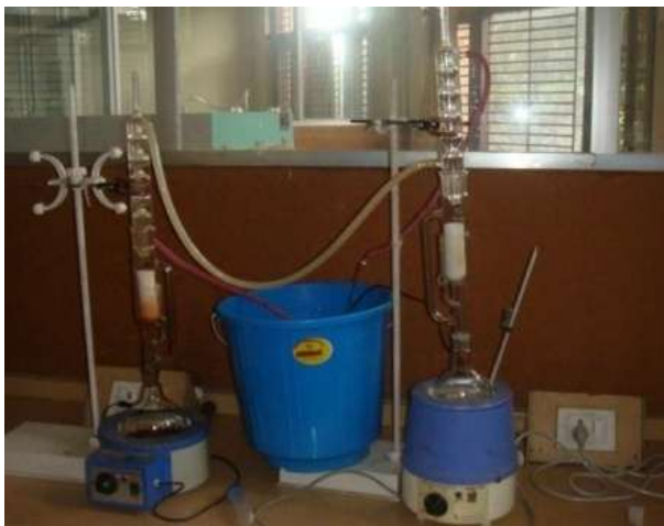
Fig: soxhalation of plant extract
